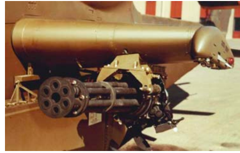
20mm Vulcan cannon mounted on Cobra winglet
