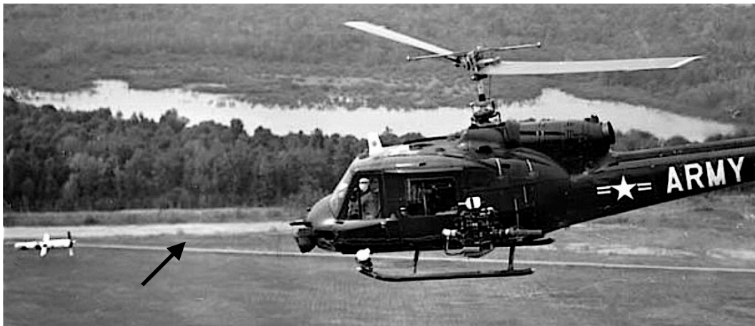
Antitank wire-guided missile just after launch from Huey (guide wire is just barely visible, see arrow)
