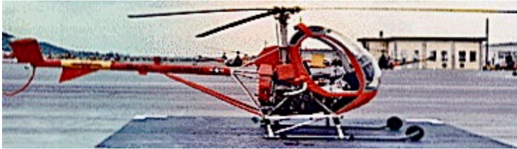
The TH-55A Osage training helicopter had a maximum cruising speed of 75 mph and a range of 200 miles.
