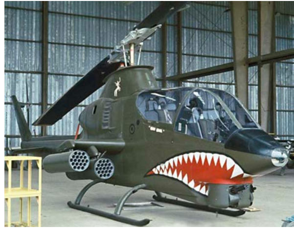
Cobra helicopter showing two XM159 19-tube 2.75-inch rocket pods attached to its right wing
