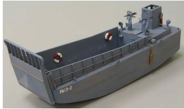
An LCM-3 Mike Boat model LCMs were bigger than Higgins boats and made mostly of steel instead of wood.
