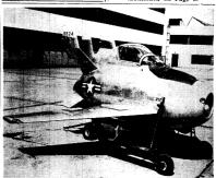
PARASITE JET, designed to operate from the bomb-bay of a large bomber, take off and land in mid air, thus affording protection to the mother ship from attacking enemy fighters, is known as the XF-85. It will be one of the jets featured in the air show to
