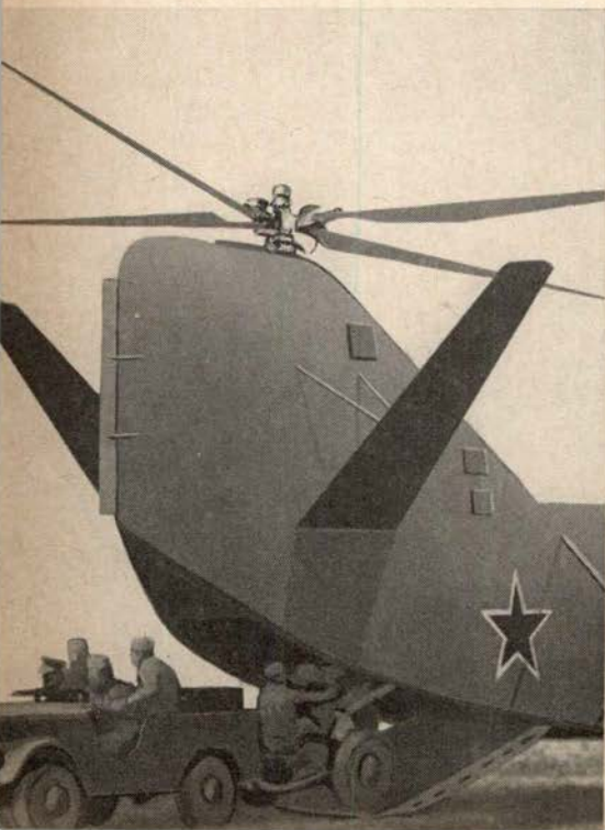
Figure 14. Vehicles and artillery pieces can be driven up a ramp into the Horse.
