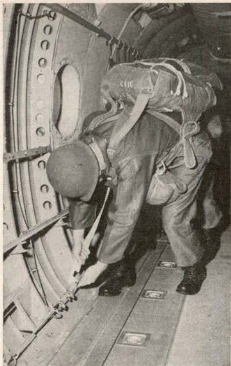
Figure 3. A modification near the floor of the H-21C provides an anchor line to which the trooper "hooks up."
