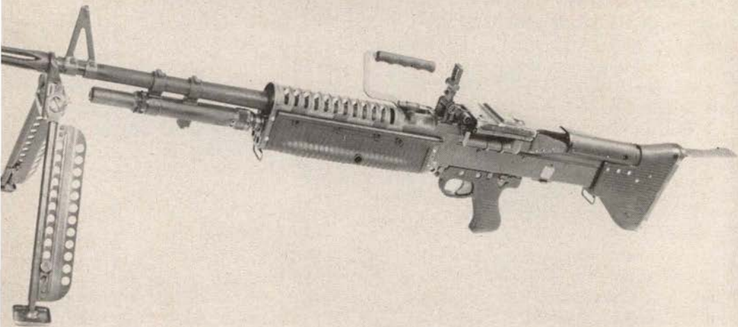
Figure 4. The M-60 machinegun on bipod.
