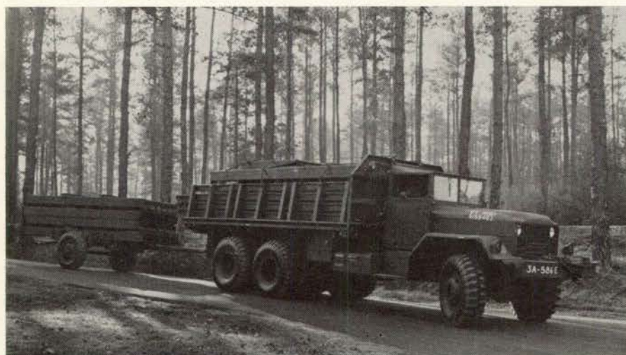
Three of these 23-ton trucks carry the Infantry division's 114 feet of fixed bridge. A floating bridge company with 730 feet of class 60 bridge (see photo preceding page) requires 60 of these trucks and 2525 gallons of fuel to move 100 miles.
