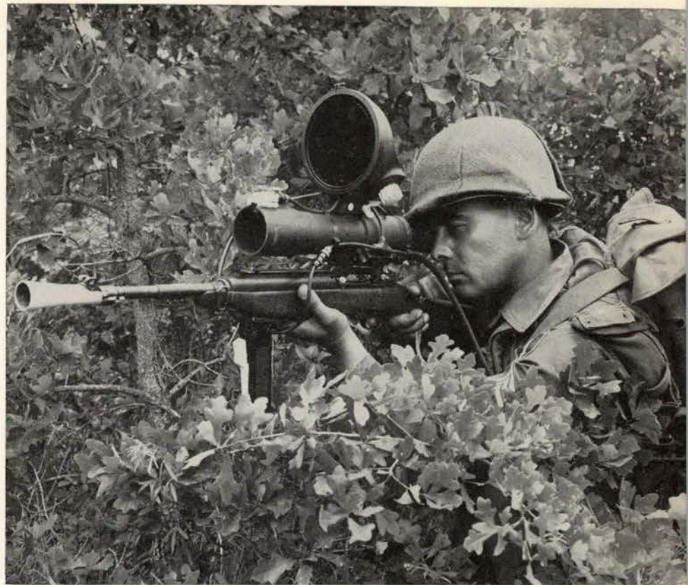
Figure 1. T-1 infrared sight mounted on the carbine.
