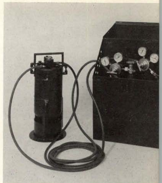
Figure 3. The Artillery Simulator operates on the same principle as the Gunfire Simulator. Considerably safer than an explosives-type device, it produces realistic sound, smoke and flash. It can be used to the rear of as well as forward of troops. The simulator motor is not shown in the illustration.
