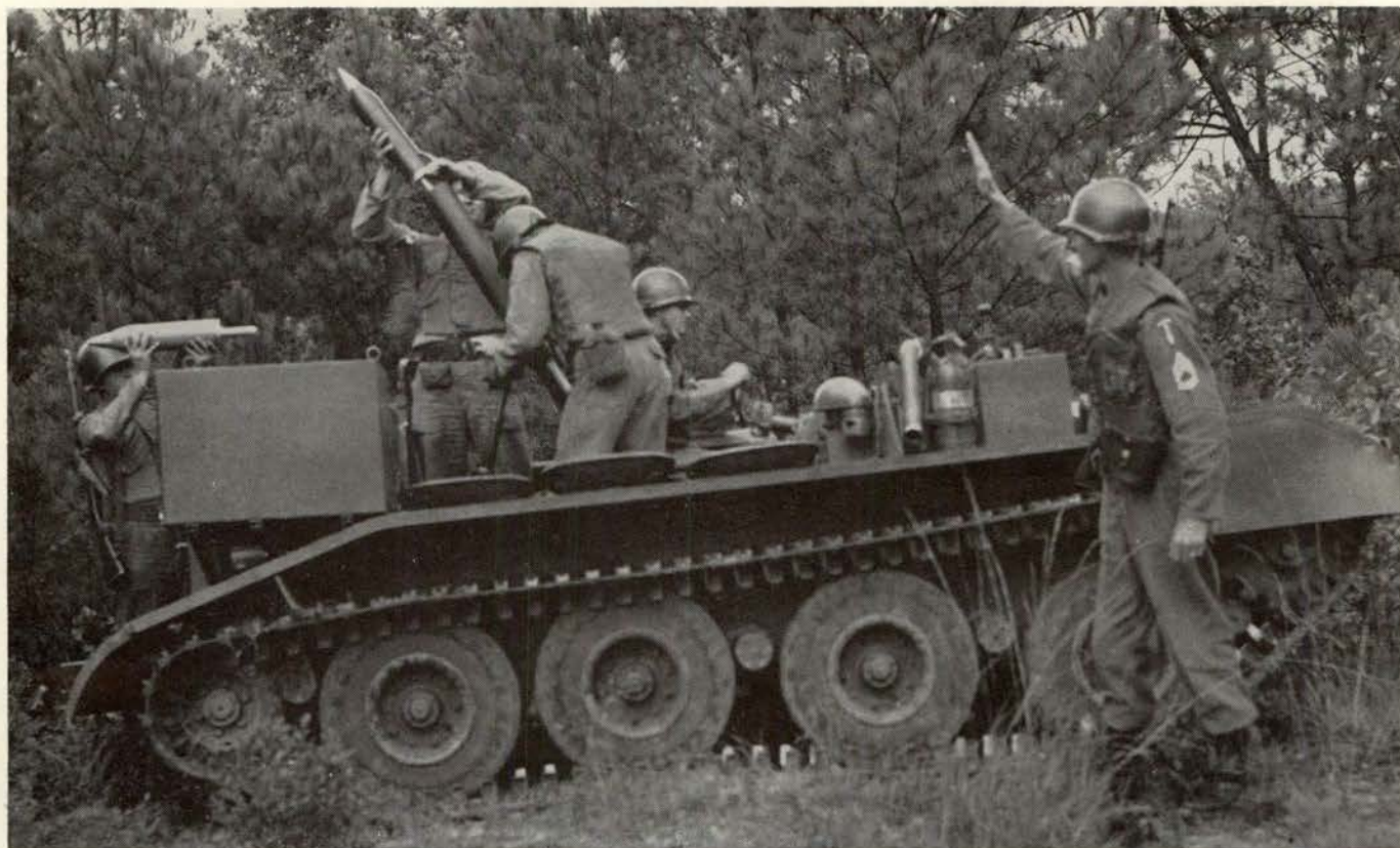
Side view of the 4.2-inch mortar mounted on the M56 carriage. Note ammunition stowage boxes and seats for crew.
