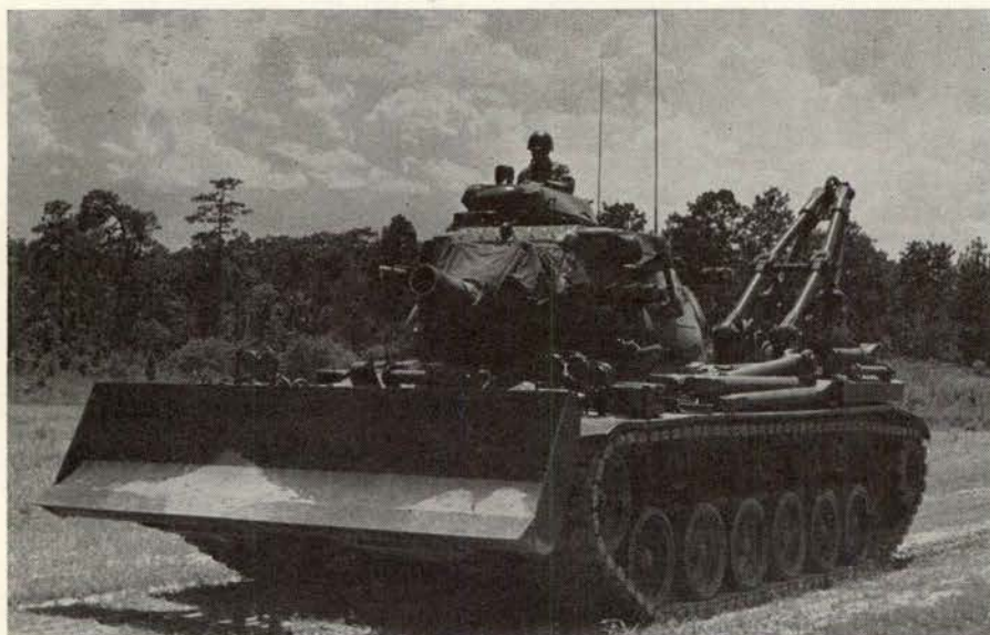
This heavily armored combat engineer vehicle (CEV), three of which are in the Infantry division, is considered a must for clearing obstacles and "bunker-busting" while under fire. Weight: over 54 tons. Fuel consumption: over two gallons per mile on good roads.
