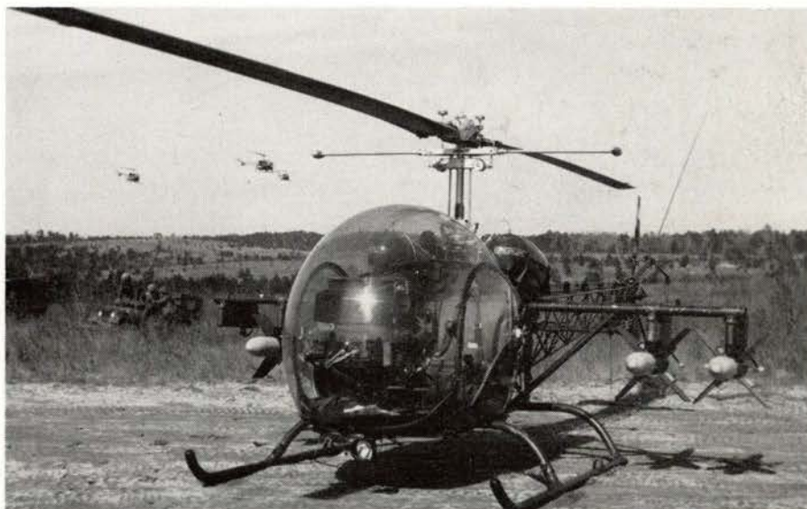
Helicopter-mounted SS10s combine Infantry's antitank missile firepower with air mobility. The rugged, adaptable SS10 system offers many possibilities of imaginative employment in a variety of roles.
