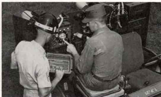
Launch procedures get careful emphasis as students apply a checklist printed in the circuit-tester cover. The circuit-tester checks for malfunctions and control.
