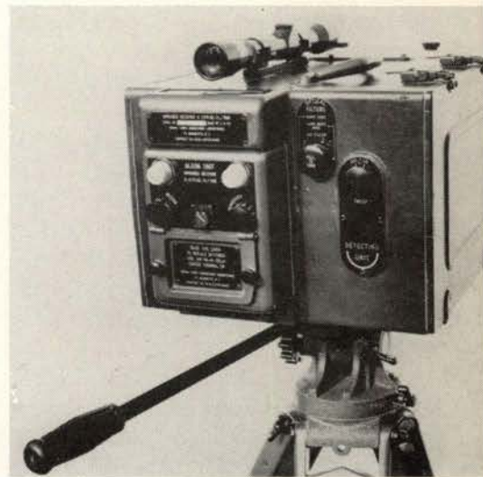
Figure 6. Infrared intrusion detector.
