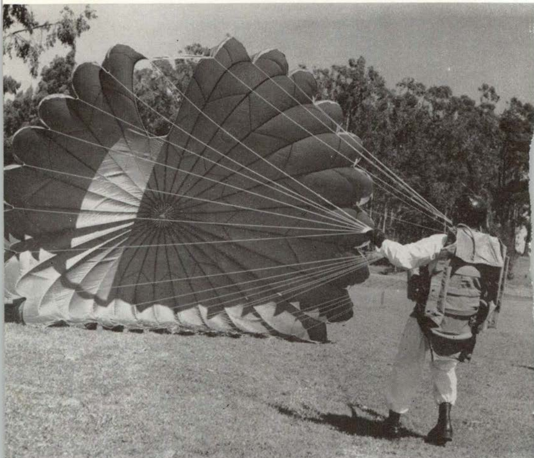
The canopy is collapsed after a free fall jump. Note the open gore.
