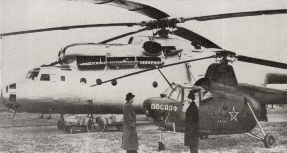
A huge, new helicopter, the HOOK is shown here with the Soviet HARE. It is powered by twin gas turbines.
