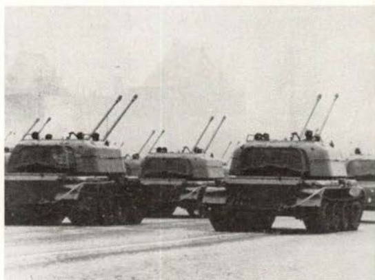
A twin 57mm antiaircraft gun mounted on a full-tracked medium tank chassis.
