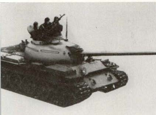
The new Soviet T-54 tank which combines a lower silhouette and improved slopes and surfaces with the best features of their T-34.
