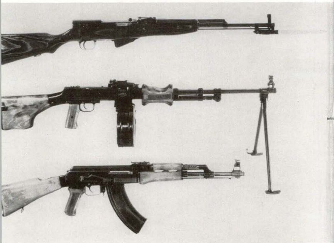
New family of Soviet small arms all of which fire a 7.62mm round. Top : rifle. Center : light machinegun. Bottom : submachinegun.
