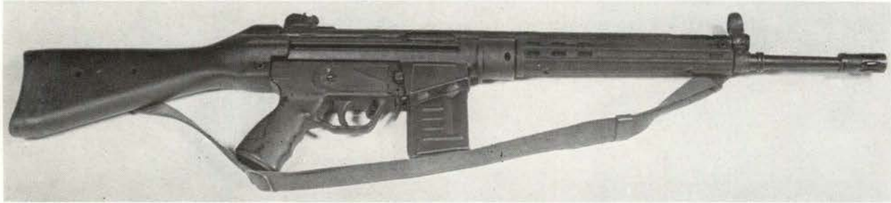
Figure 1. The H&R G3 (M) Rifle (right view). CHARACTERISTICS: Overall length, 36.1 inches; overall weight (combat loaded) approximately 8 pounds; ammunition fed from 20-round detachable straight box magazine; Cyclic rate of fire, approximately 600 rpm.
