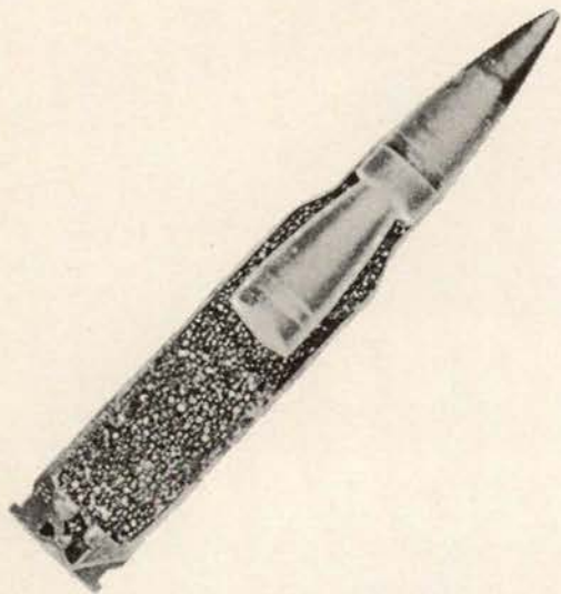
A cross-section of the Duplex M198 shows the cant of the rear bullet which causes its dispersion.
