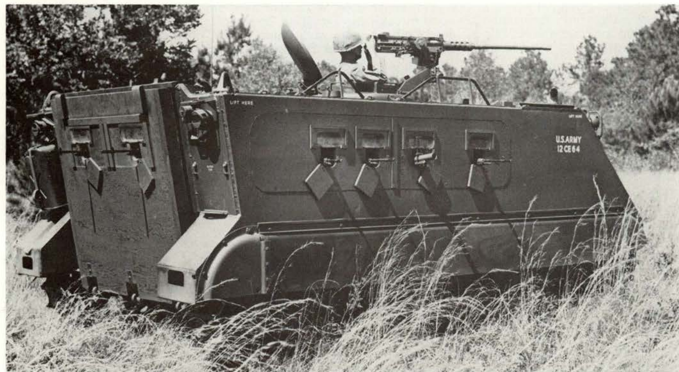
The modified M113 armored personnel carrier with firing/observation ports open.
