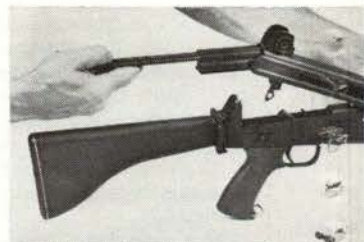
Right. Removing the operating parts.
