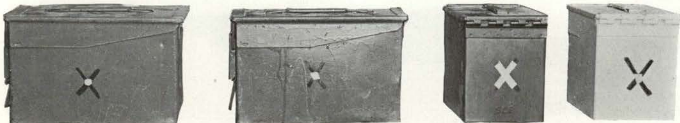
Targets used in the penetration tests were four government-issue ammunition cans filled with water. Top photo shows entry side of cans prior to tests marked with an "X" to designate the aiming point. Lower photo shows exit sides of cans after the test. From left to right in top photo: Can engaged by 7.62mm round through short axis; can engaged by 5.56mm round through short axis; can engaged by 7.62mm round through long axis; can engaged by 5.56mm round through long axis. Lower photo shows cans (after test) in reverse order, from left to right. (All cans were engaged at 25 meters)
