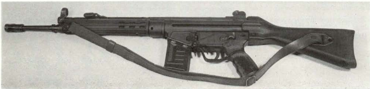
Figure 2. The H&R G3 (M) Rifle (left view). Note the unusual location of the operating handle (left front portion of the operating rod tube mounted over the barrel).
