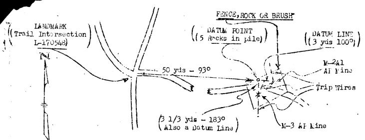
l. It may be necessary to have more than one Datum Point for the same field. This is permissable if both Datum points are referred to the same landmark by Direction and Distance.
