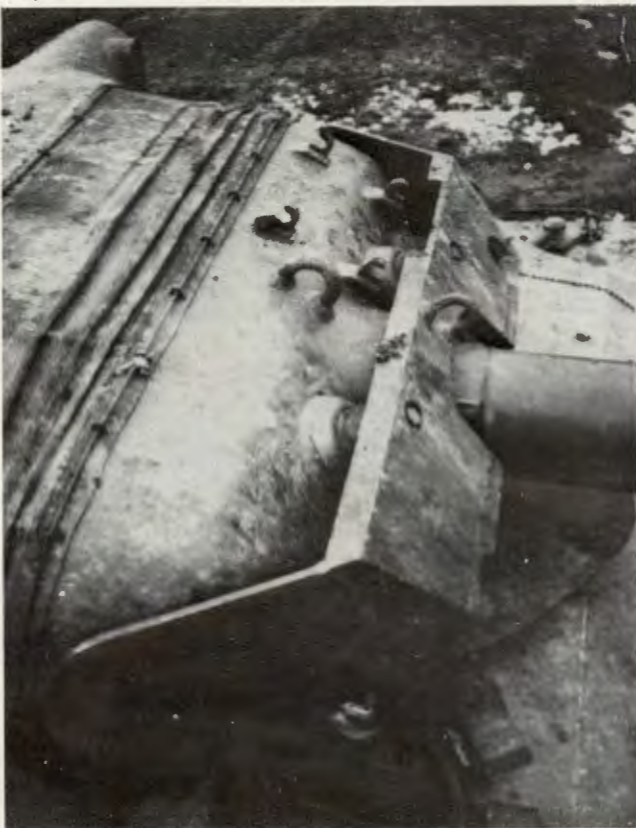
Right side of the gun mantlet, showing the armor protection added. Note rubber shock absorbers on either side of the gun tube on which the armor is mounted.
