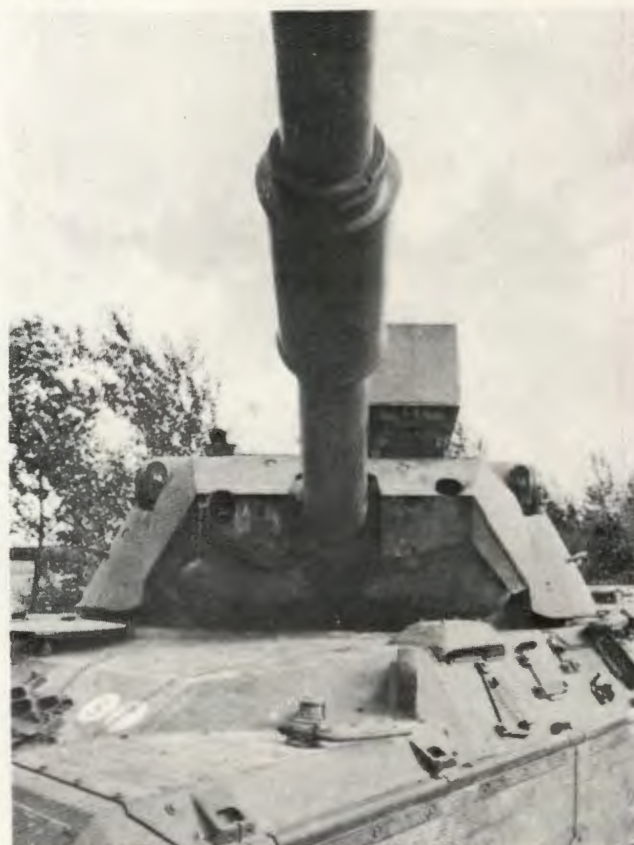
Front view of gun mantlet, showing the additional protective armor.
