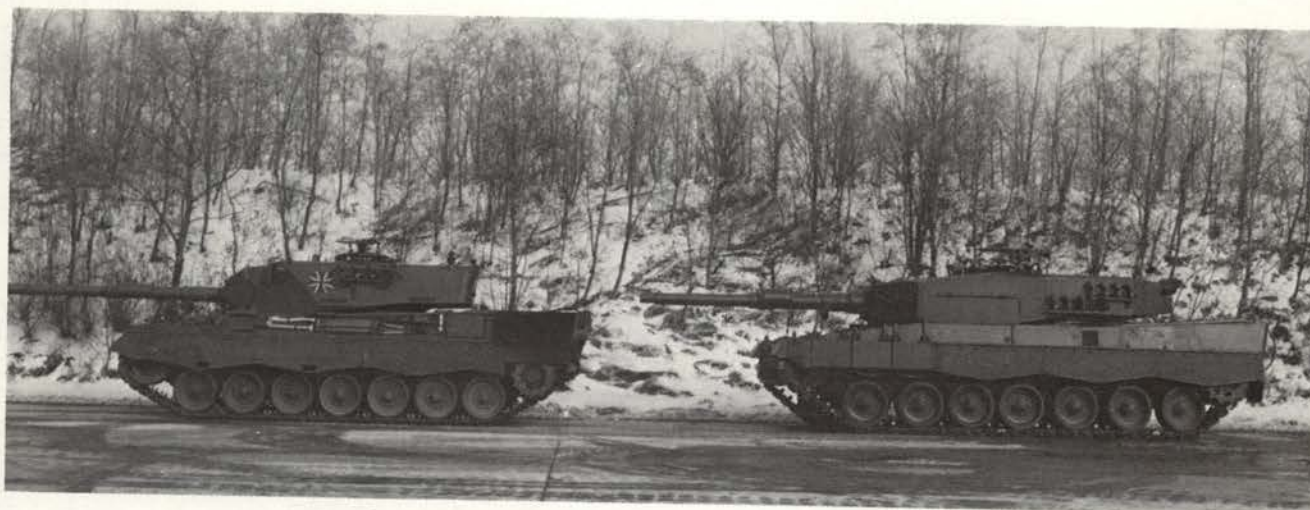
A Leopard 1 (left) and a series configuration Leopard 2 (right) illustrate the differences between the two MBTs.
