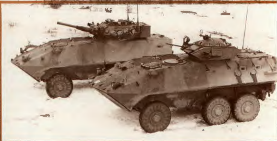
Two of the three versions of the Canadian general purpose armoured fighting vehicle are shown here. Three views of the Cougar appear at left, above, and center. The Grizzly is at the lower right. Note the gun ports adjacent to the vision blocks in the rear third of the Grizzly's hull.
