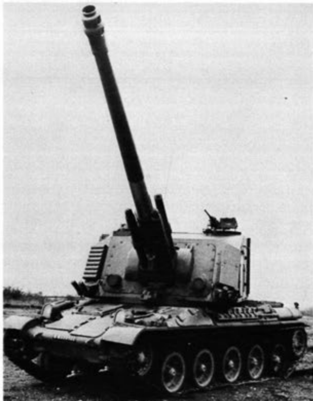
The 155mm GCT Self-Propelled Gun is mounted on an AMX30 chassis. It is currently undergoing test by the French Army.
