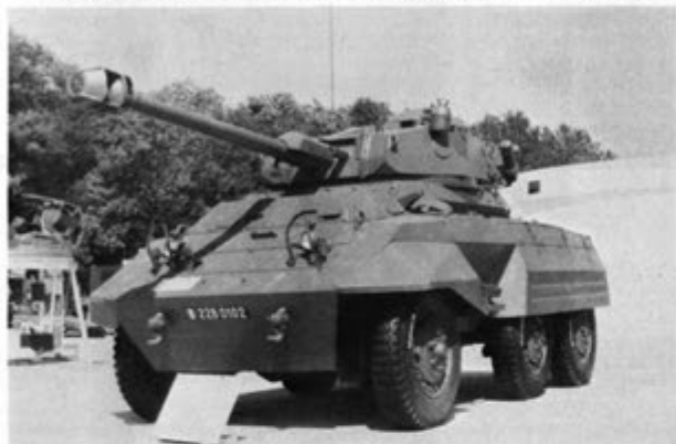
American M20 utility vehicle fitted with AML90 turret mounting a 90mm gun, a 7.62mm machine gun and smoke dischargers.
