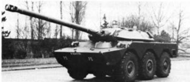
The AMX10RC uses AMX10P components and is armed with a 105mm gun.
