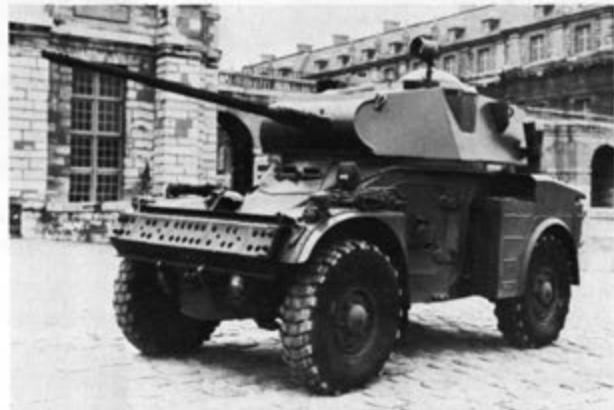
The AML30 is armed with a turret-mounted 30mm cannon and carries 200 rounds of ammunition for the gun.
