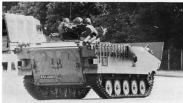
The AMX10P mounts a 20mm cannon and a 7.62mm machine gun.
