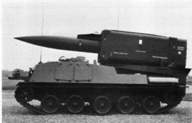
AMX30 fitted with Pluton tactical nuclear weapon system.
