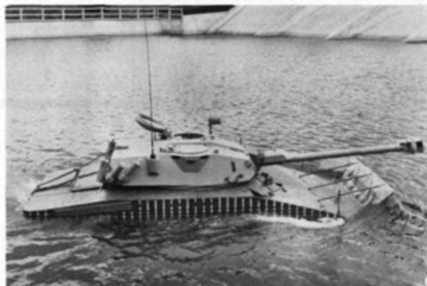
The AML90 equipped with the Panhard-designed flotation kit.
