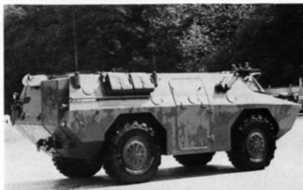
The four wheel drive Berliet VXB was designed primarily to fill the requirement for an anti-riot vehicle for the French Police.
