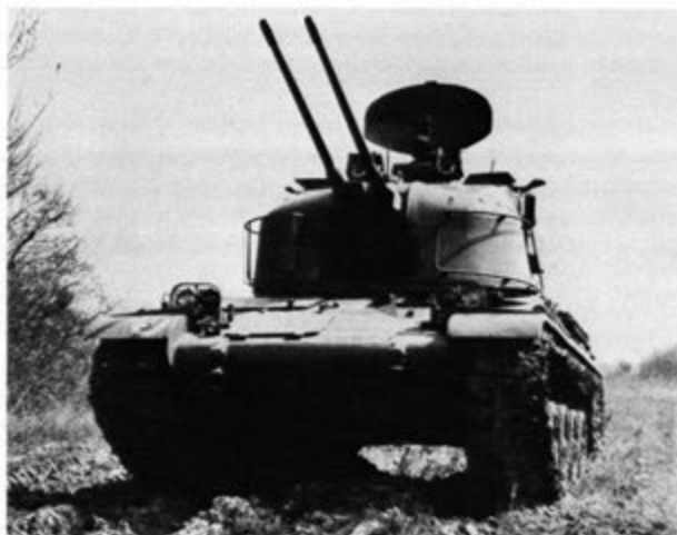
The AMX30 Antiaircraft Tank is fitted with a turret armed with two 30mm guns and the DR-VC-1A radar. The guns have an effective range of 3,000 meters and can fire 650 rounds per minute per barrel.
