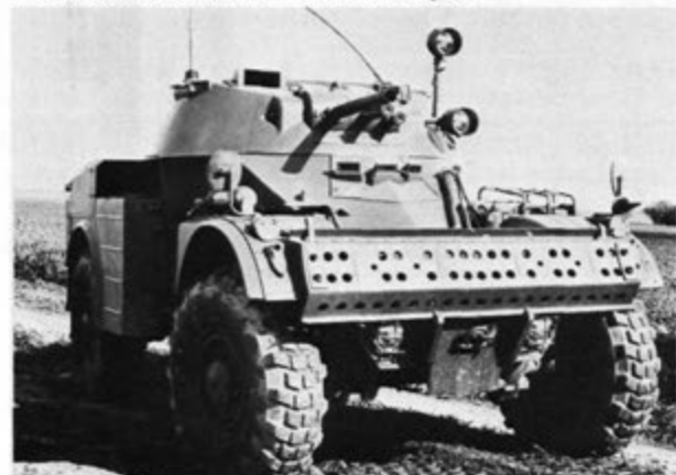
The AML60-7 mounts a 60mm breech-loaded mortar.
