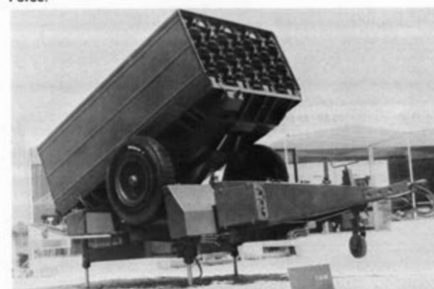
The 21 rockets of the RAP14 system have a range of nearly 10 miles.
