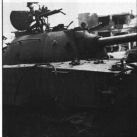
Most 105mm howitzers had 2-3 rounds of HEAT at the gun positions on 12 May. Probably a HEAT round through the turret disabled the PT76 which was later destroyed by M72 fire.
