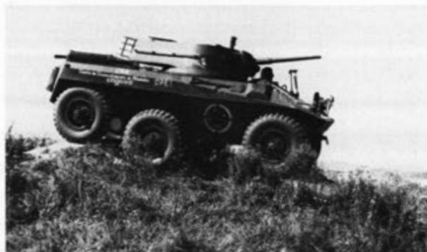
The CRR wheeled reconnaissance vehicle will replace the US M8 armored cars and the M3A1 light tanks in the Brazilian Army. Specially designed tires enable the vehicle to travel considerable distance at normal road speed when perforated by bullets.
