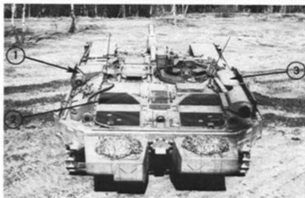
① Gas turbine air cleaner; ② Cooling air inlet; ③ Diesel engine silencer.
