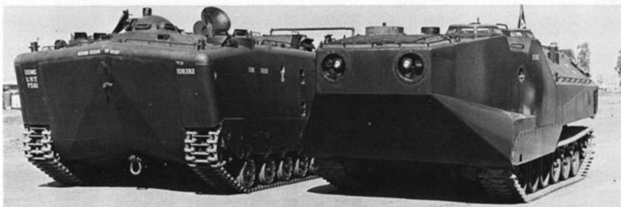
The LVTP5, left, could maintain 6.8mph in water by track propulsion alone. The LVTP7, however, can reach higher speeds through the use of water jets.
