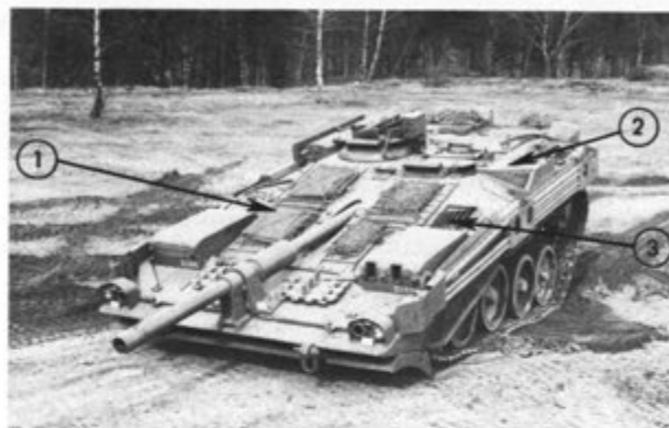
① Diesel engine combustion air inlet; ② Gas turbine air inlet; ③ Gas turbine exhaust.
