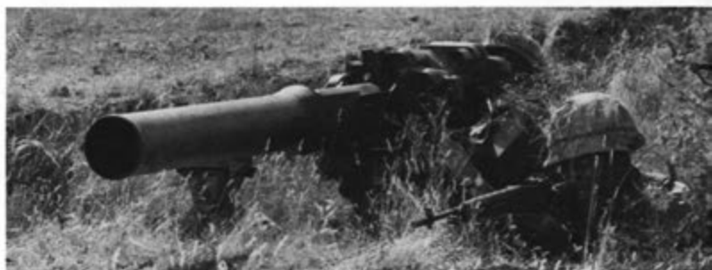
The TOW missile system is a tube-launched, optically-tracked, wire-guided system capable of penetrating all known tanks at greater than 3,000 meters.
