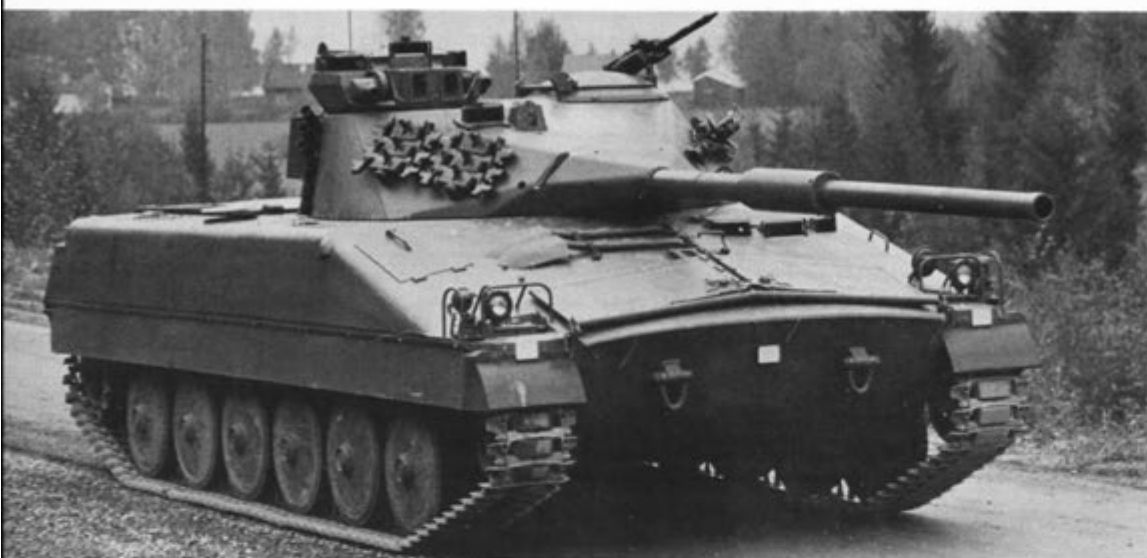
The Swedish IKV91 , which weighs only 15 tons and possesses low ground pressure giving it good traction in wet going, carries a 90mm Bofors low-pressure gun.
