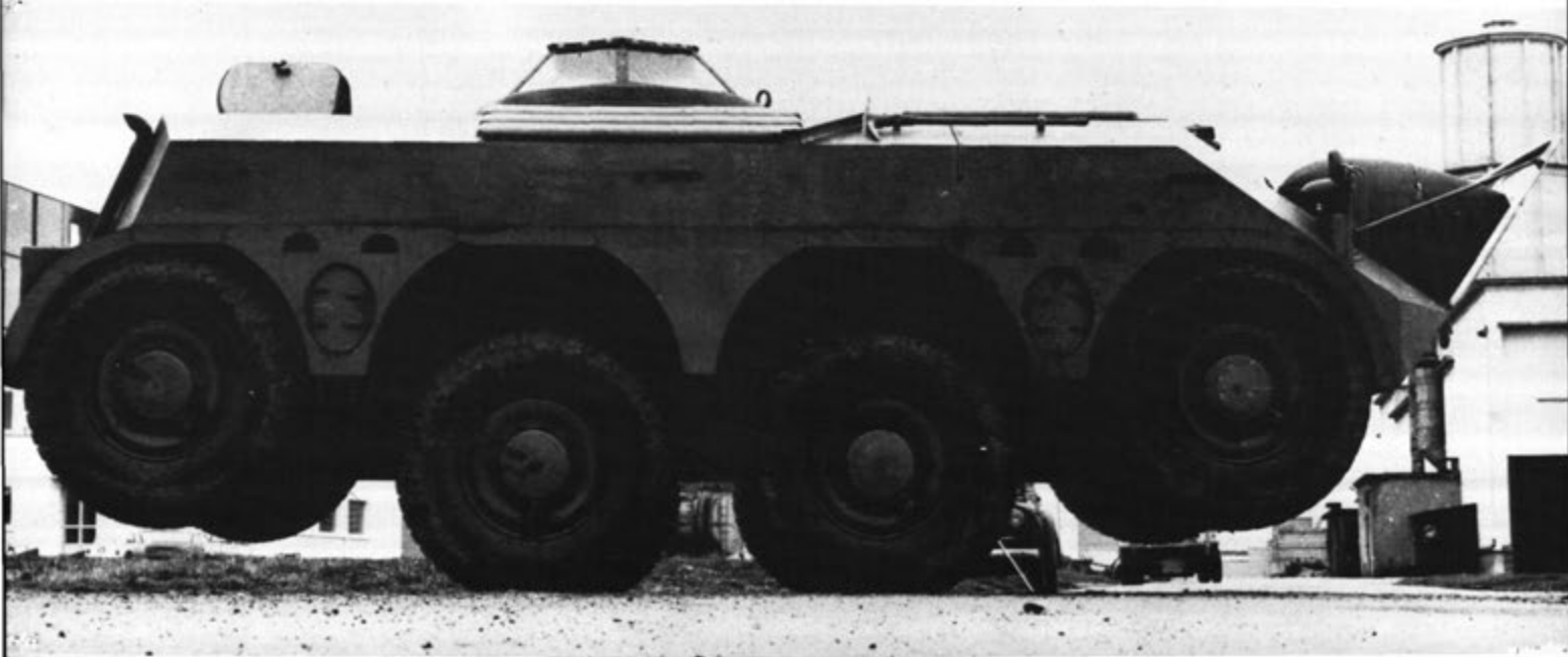
Panhard M2 with its front and rear pairs of wheels raised off the ground for a pivot turn.
