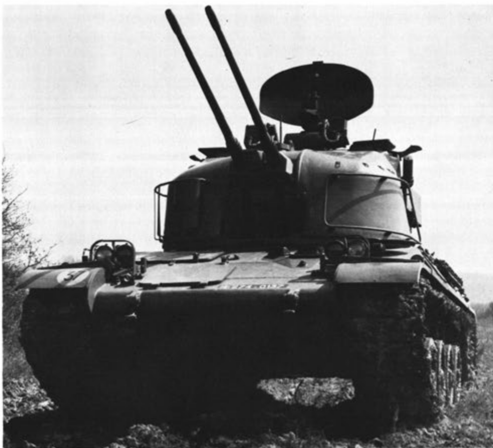
AMX30 anti-aircraft tank with two radar-controlled 30mm automatic guns.
