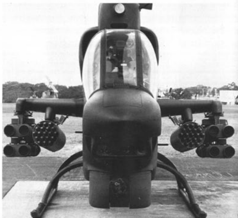
The front view of the KingCobra shows the variety of armament it can expend, including three-barrel 20mm cannon in turret and rockets, and antitank missiles on wing stores.
