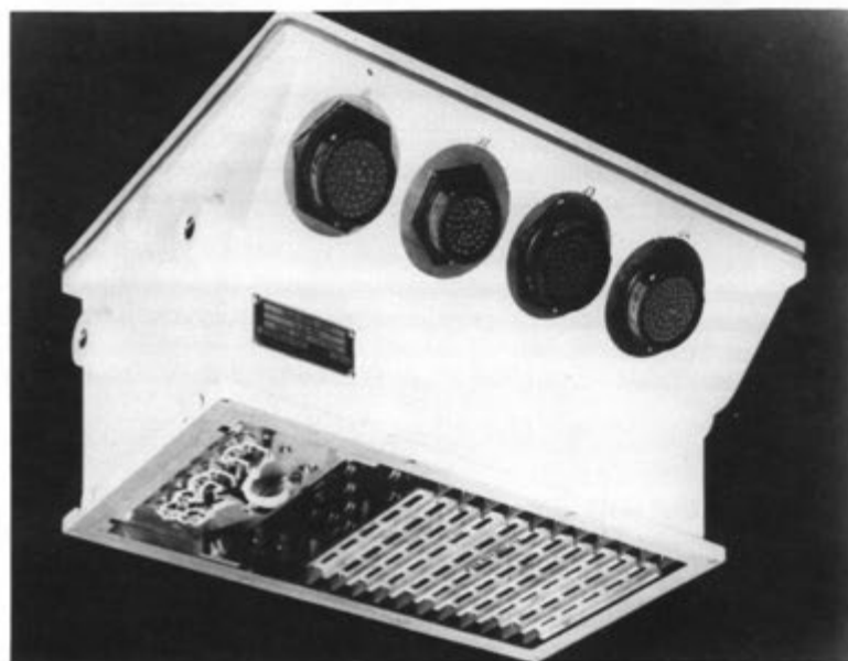
Ballistic computer with bottom cover plate removed.
