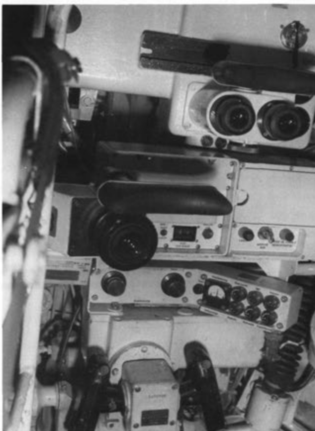
The system installed in a Leopard tank. Top, laser and sights; center, gunner's control units and emergency telescopic sight; bottom, gun elevation and turret traverse controls.
