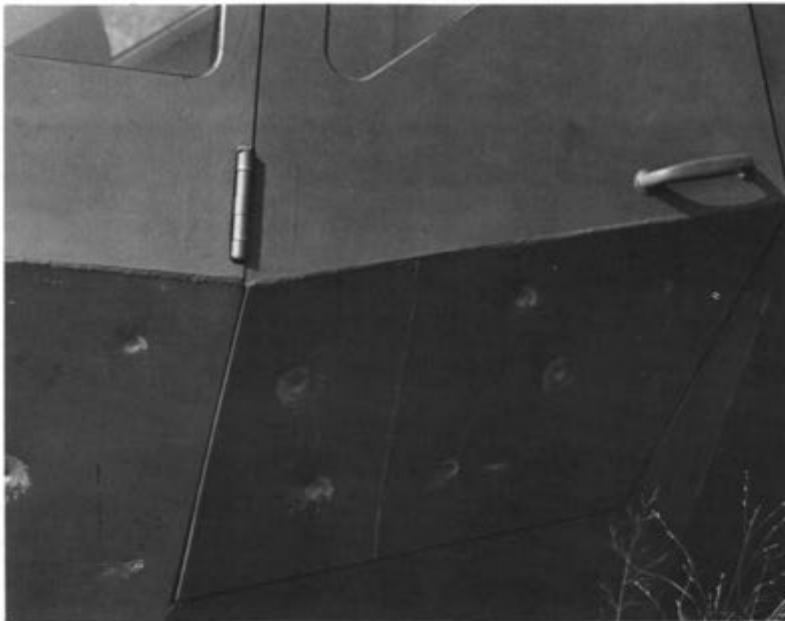
The fuselage of the mock-up of an AARV was hit with a .30 caliber ball and armor piercing ammunition at zero degrees and 30 degrees obliquity. Only denting resulted, according to Sikorsky.
