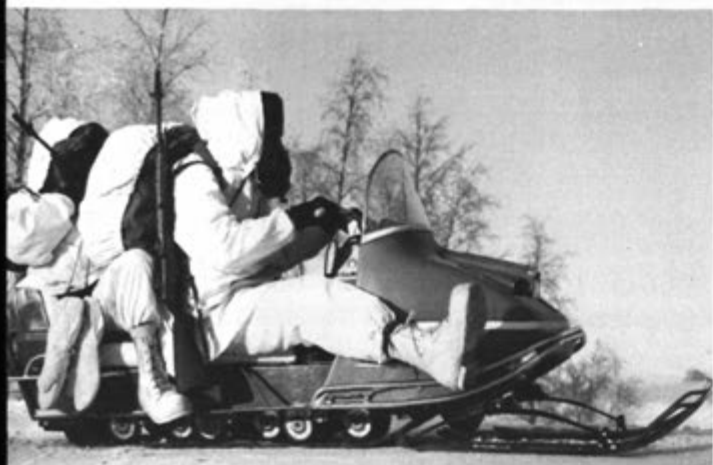
During operations last winter, the U. S. Army, Alaska, evaluated 10 snowmobiles at Fort Wainwright. Prerequisites for selection as a test vehicle were that it be capable of being lifted by two men, fit inside an M113 APC, and be able to transport two fully-equipped men over unbroken snow.
