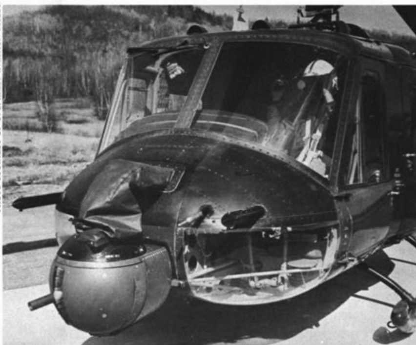
One of the highlights of the course is firing the M5 system during the qualification course program. The system launches 150 40mm grenades with a lethal bursting radius of 10 meters.
