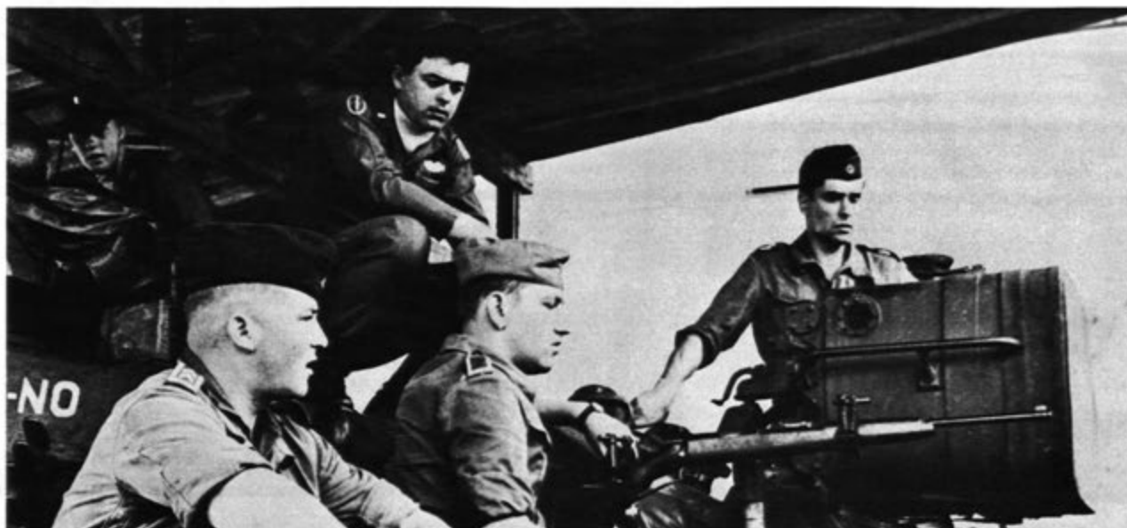
Mounting a .22 caliber rifle alongside the main gun tube enables the entire crew to engage in realistic training exercises without moving their tanks off post.
