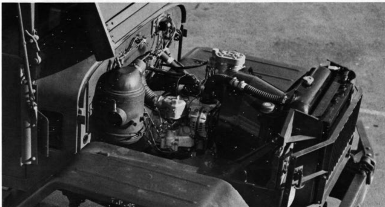
The 185 horsepower, 5000 rpm vehicular version of the RC2-60 engine installed in a US Army M35 2½ Ton Truck.
