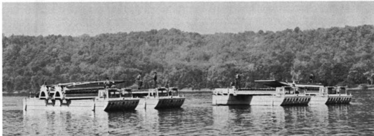
The Mobile Floating Assault Bridge under test by the Armor and Engineer Board. The MAB will support 60-ton loads when employed either singly as a ferry or as a bridge element. As a ferry it can move at 8 mph with a full load. Interior bay unit roadway segments of each vehicle are 26 feet long.
