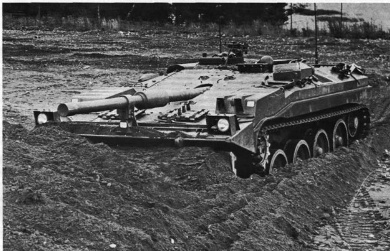
S tank excavating a firing position with its bulldozer blade
