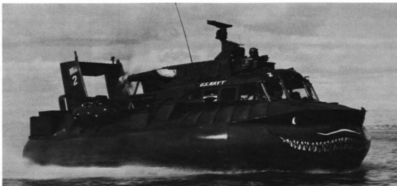
A heavy ACV skims over San Francisco Bay following overhaul after eight months of service in Vietnam. Modifications included installation of auxiliary fuel tanks, addition of communications equipment, new skirts for improved performance and ease of maintenance, and "puff ports" for improved directional control.
