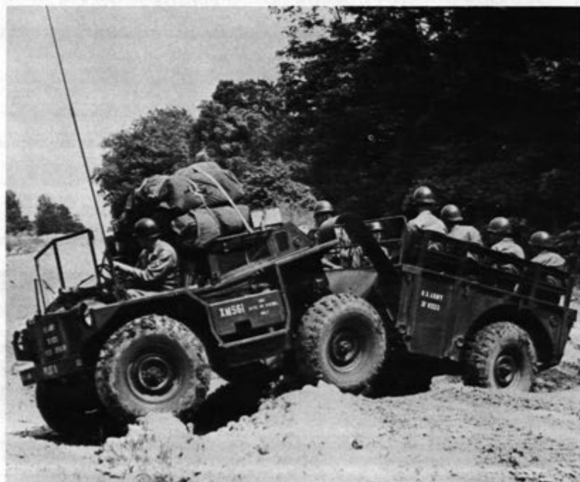
The XMS61 Gama Goat, a 1.5-ton cargo carrier being tested by USAARENBD. The Gama Goat's two bodies are connected by an articulated joint which allows them to follow the surface of the terrain and keep all six power-driven wheels on the ground.
