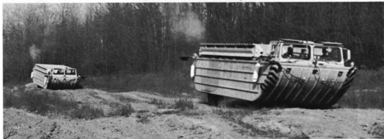
The Mobile Floating Assault Bridge under test by the Armor and Engineer Board. The MAB will support 60-ton loads when employed either singly as a ferry or as a bridge element. As a ferry it can move at 8 mph with a full load. Interior bay unit roadway segments of each vehicle are 26 feet long.
