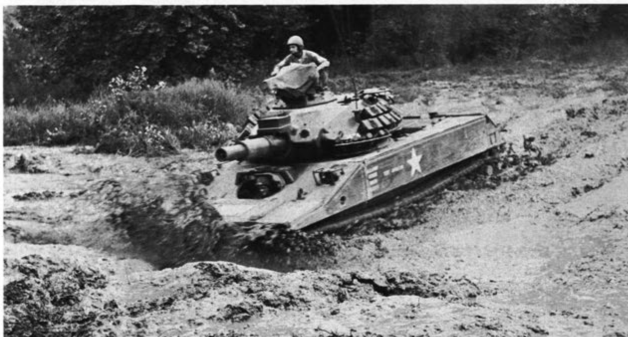
Field testing of the equipment is done by average MOS-qualified soldiers. Tests are made under conditions simulating those in which the equipment is expected to operate. Here the M551 Sheridan plunges through a mud hole.
