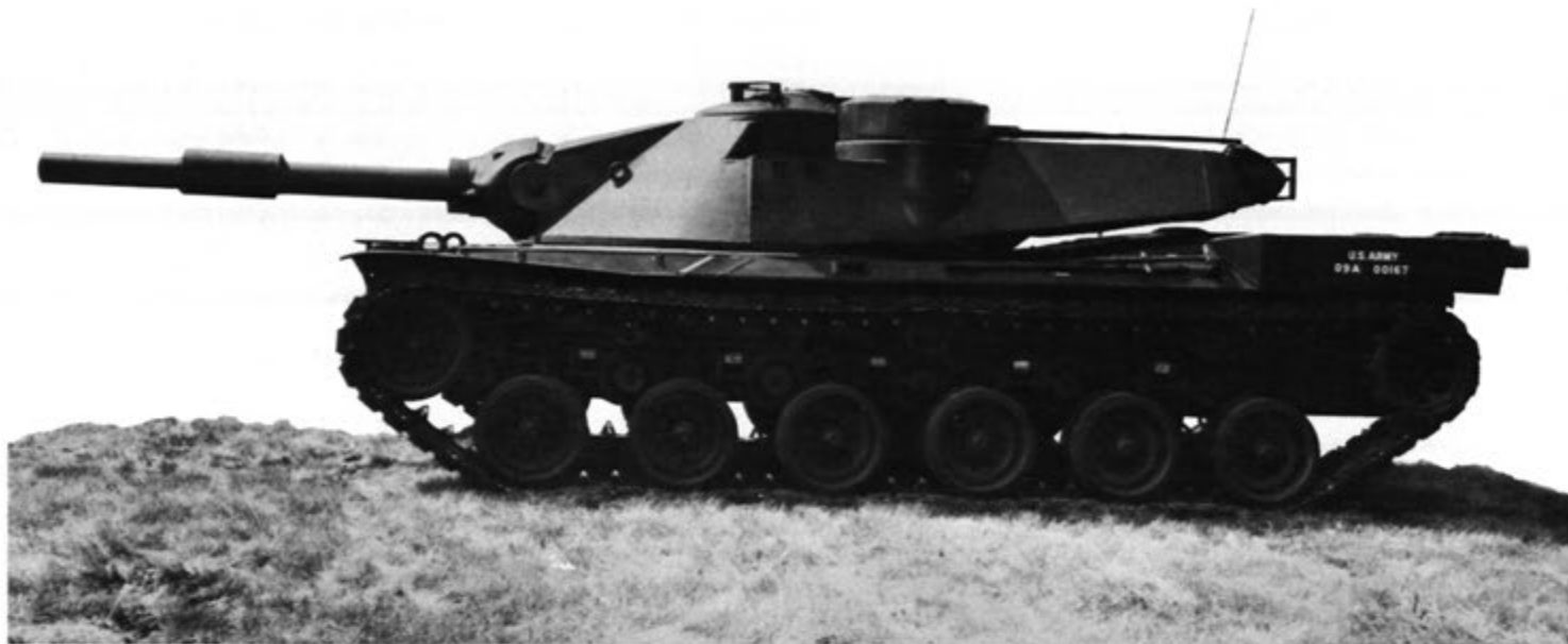
A hydropneumatic suspension allows the height of the MBT to be varied while the tank is moving.
