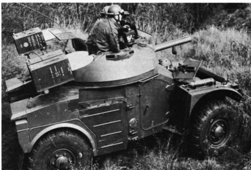
Figure 8—Four ENTAC antitank guided missiles add long range antitank capability to the AML.
