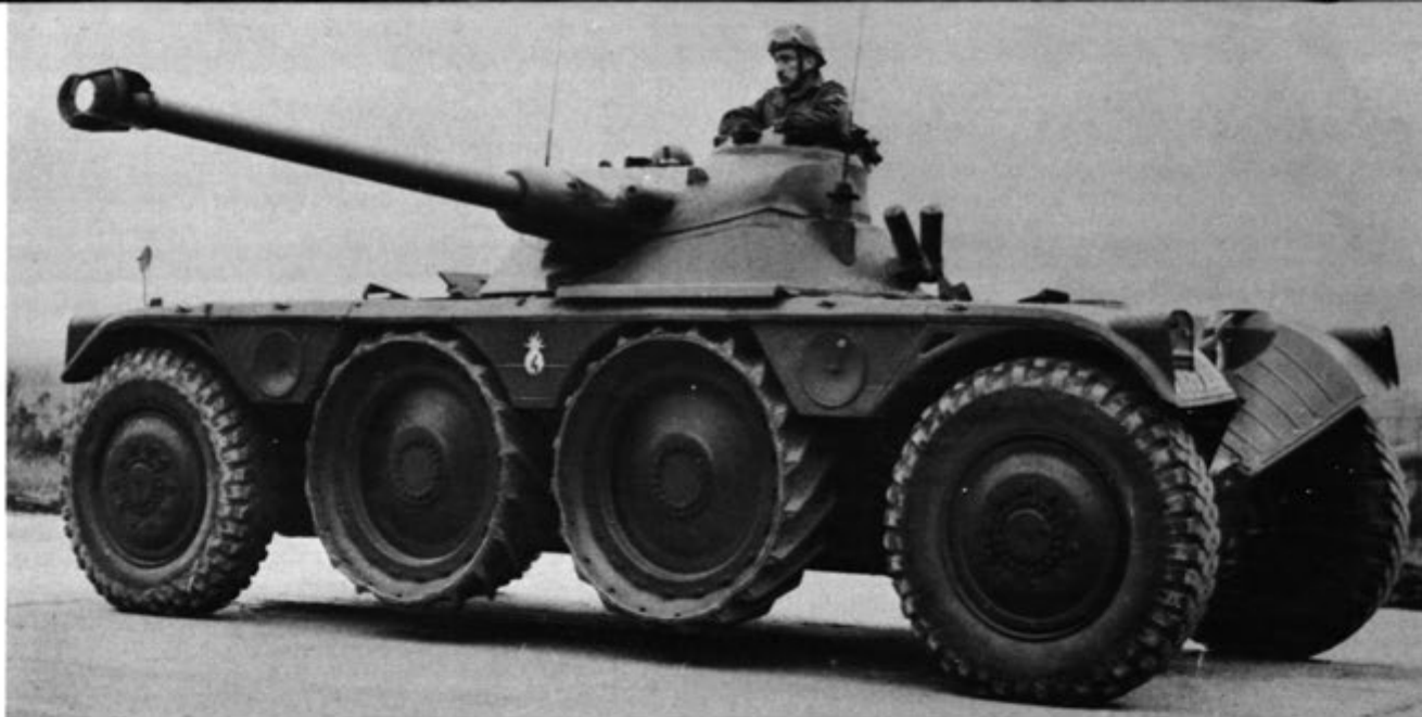
Figure 3—Original version of the Engin Blindé de Reconnaissance with FL 11 turret mounting 75mm gun. Intermediate road wheels are raised.
