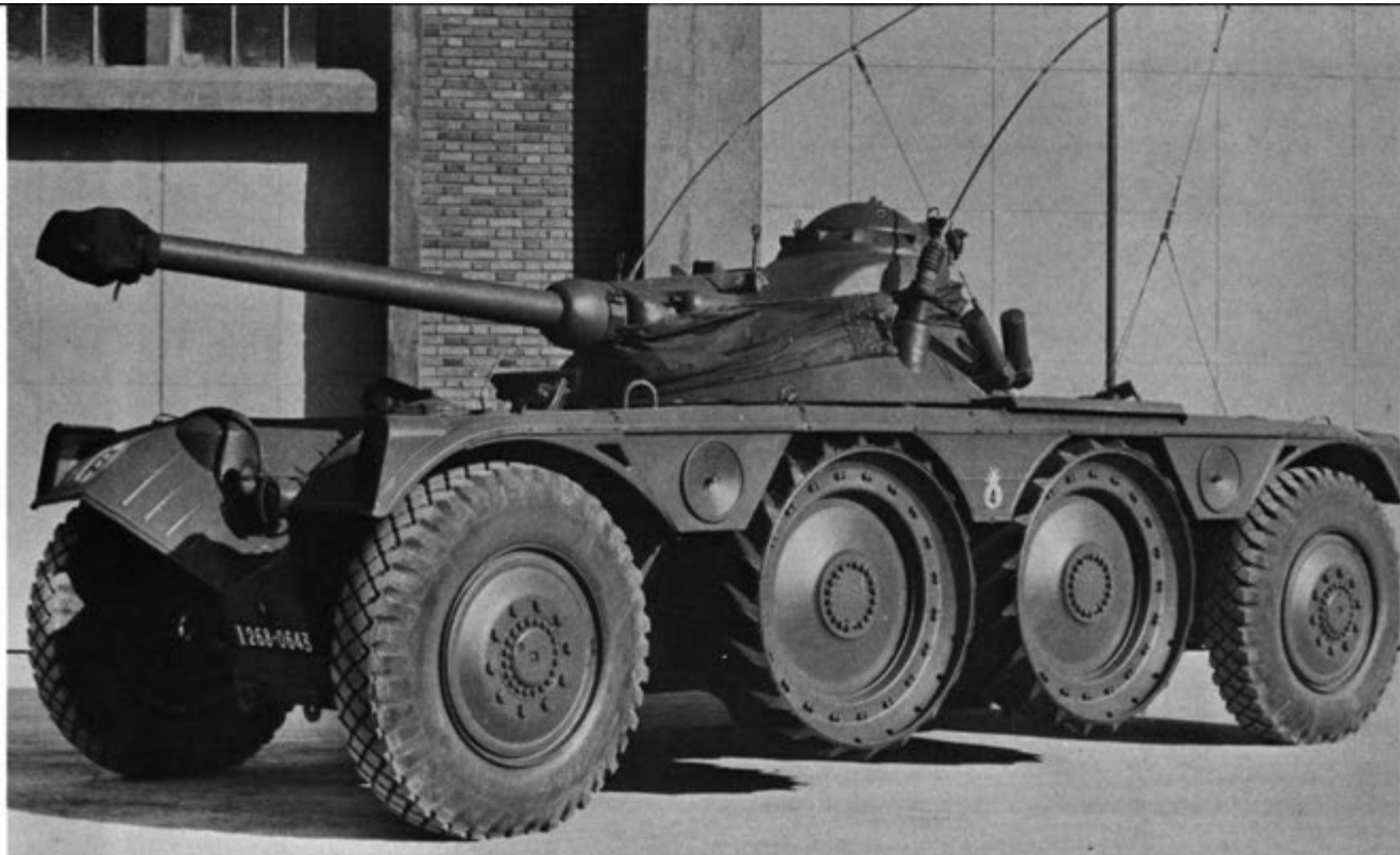
Figure 5—Latest version of the EBR with a 90mm gun permits this armored car to engage battle tanks.
