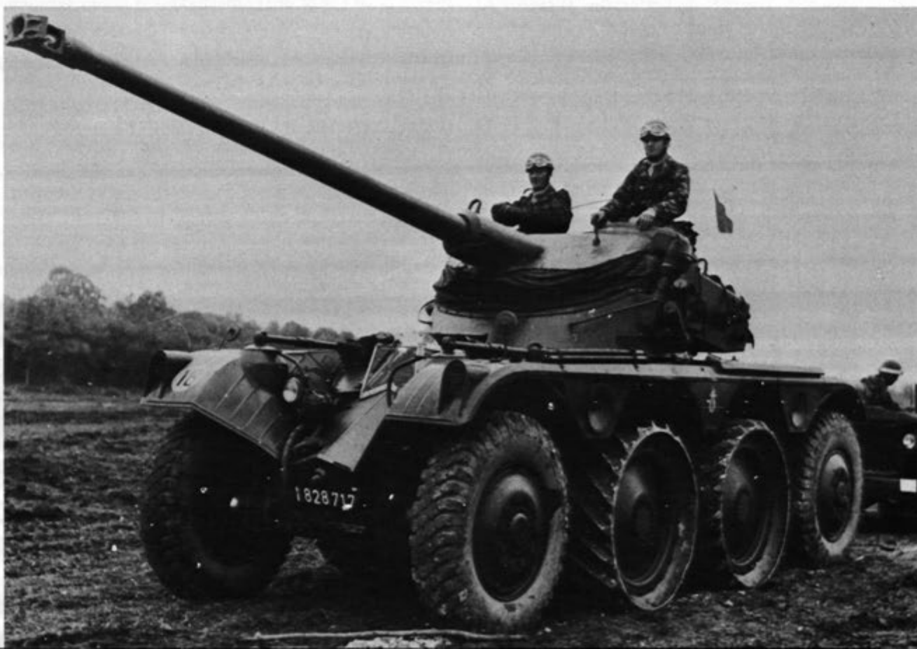
Figure 4—The FL 10 turret of the AMX 13 tank heightened the silhouette of the EBR and added weight.
