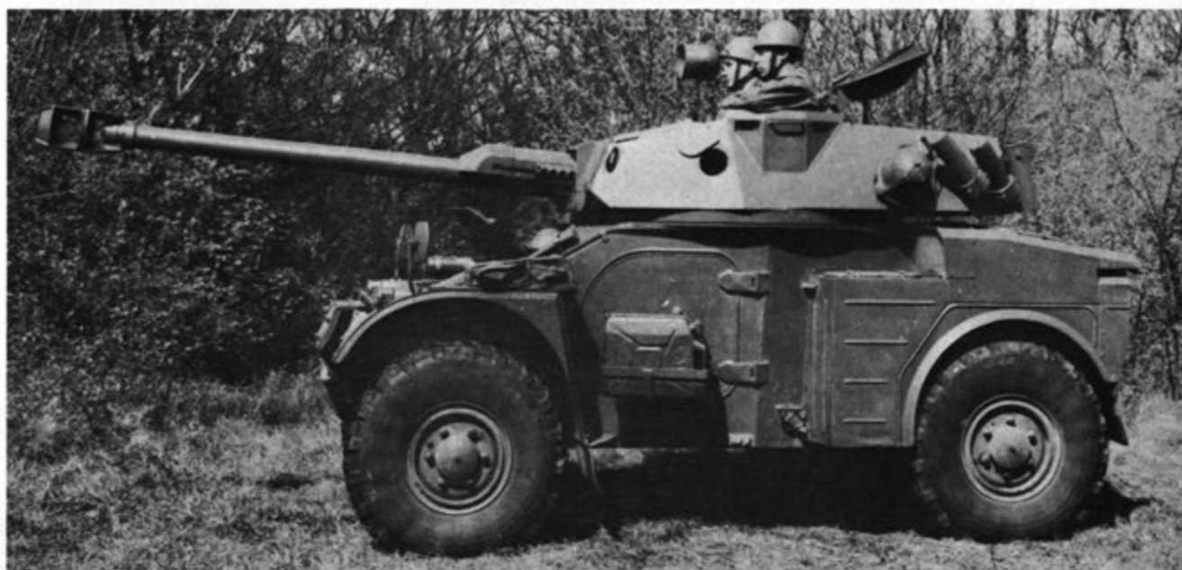
Figure 7—Second version of the Automitrailleuse Legere (AML) is fitted with a 90mm smoothbore gun and a coaxial 7.5 machinegun.
