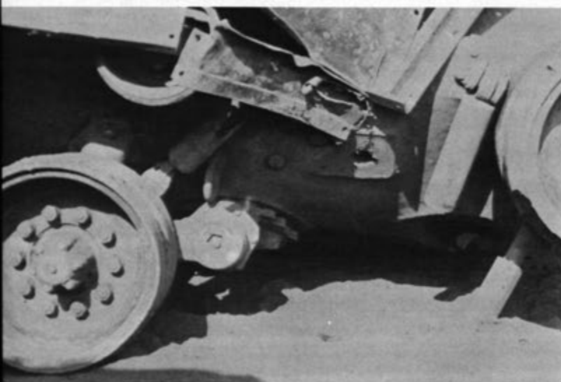
" . . . front road wheel arms sustain most of the damage."
