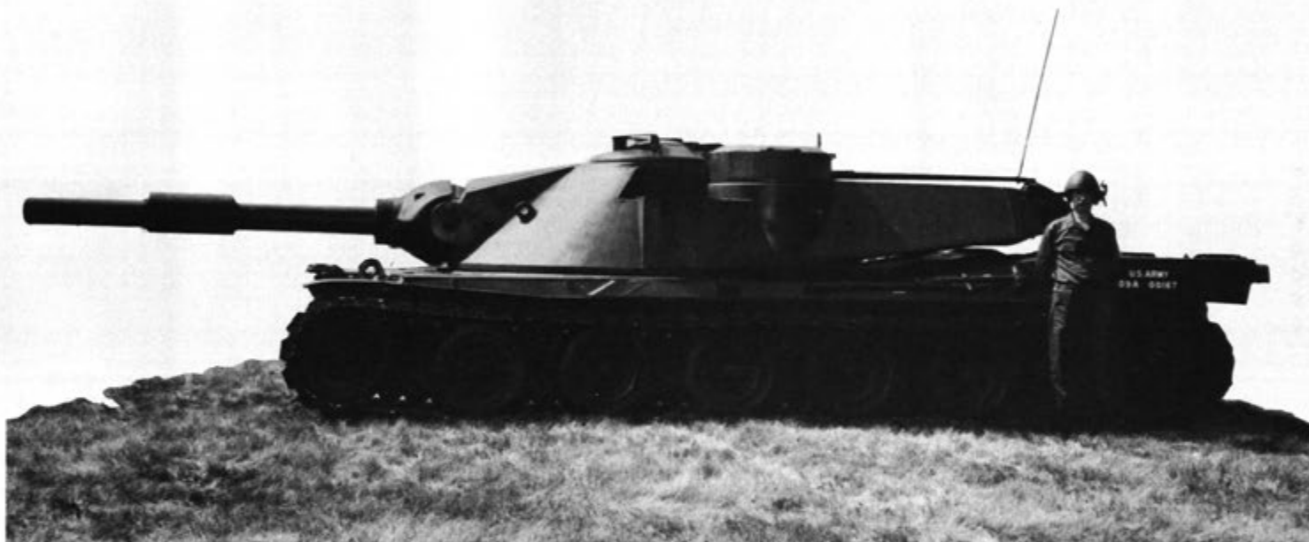
Control of the suspension is from two separate stations in the turret. Here the MBT is in the DOWN position.
