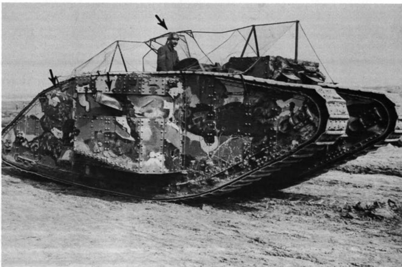
"A barren area, interlaced by abandoned trenches, torn and pocked by shell holes, and entangled throughout by seemingly endless lines of barbed wire." [Below] An early edition of the famous British Mark series. Note the arrows pointing to the well camouflaged machine guns and the unusual helmet worn by the tank commander.
