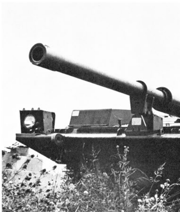
The new Swedish "S" tank has abandoned normal configuration to achieve a lower silhouette.
