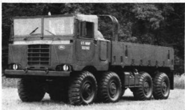
This new U. S. Army five-ton truck, the XM-656 can climb hillsides, swim streams or be airborne to remote battle areas. It is two tons lighter, more durable and requires much less maintenance than the present Army five-ton. Ford Motor Company is the designer and will perform advance production engineering for Army Tank-Automotive Command.
