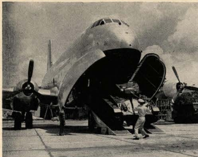
Armor—and the plane to carry it. An M24 tank is loaded on the huge Douglas C124-A. Air transport of armor is essential, is still in early stages.
