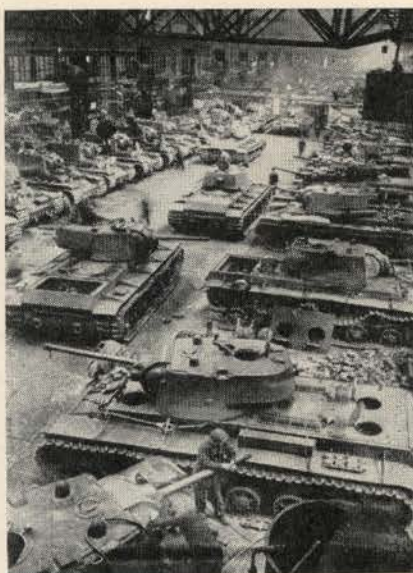
Sovfoto KV's being factory serviced at Kirov Works in Leningrad, prior to evacuation. Note plate and cast turrets.
