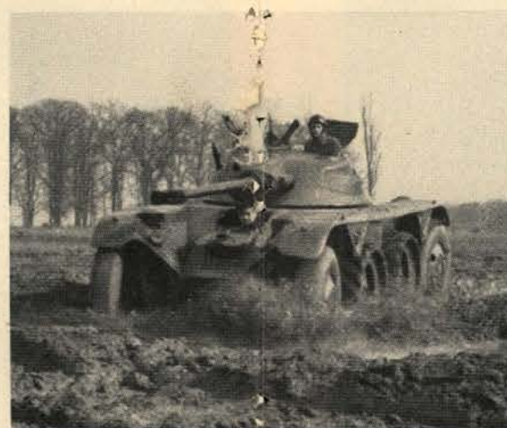
The new French armored reconnaissance car, made by the Panhard Motor Car Company, is versatile over all kinds of terrain. It weighs 12 tons and mounts a 75mm gun in a 360° turret. Crew is four and vehicle has a driver at each end, can be driven in either direction.
