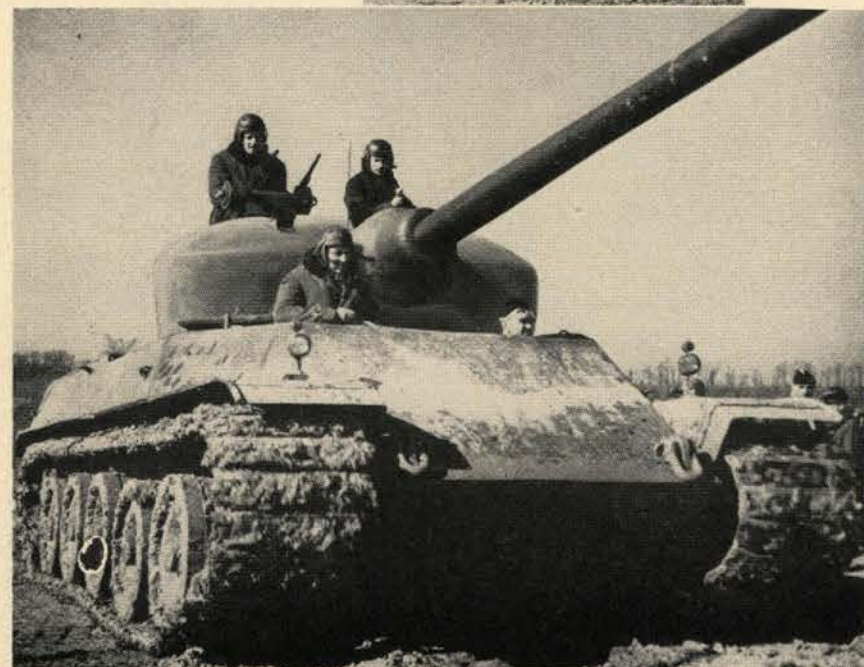
The new French heavy tank weighs 50 tons. It has a crew of four, and can mount a 100 or 122mm gun. Its 1,000 hp engine allows a maximum speed of 30 mph.
