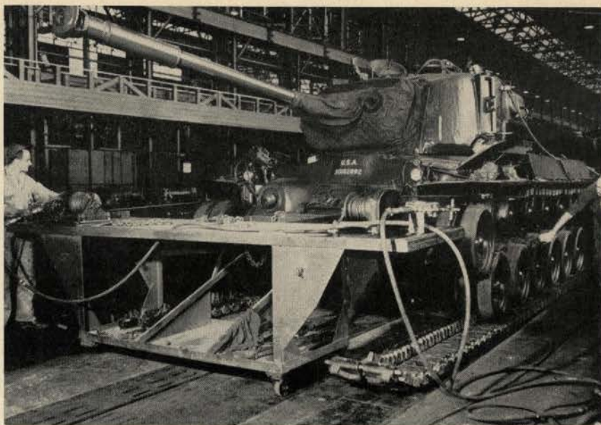
A Patton receives its tracks on the assembly line at the Detroit Tank Arsenal.
