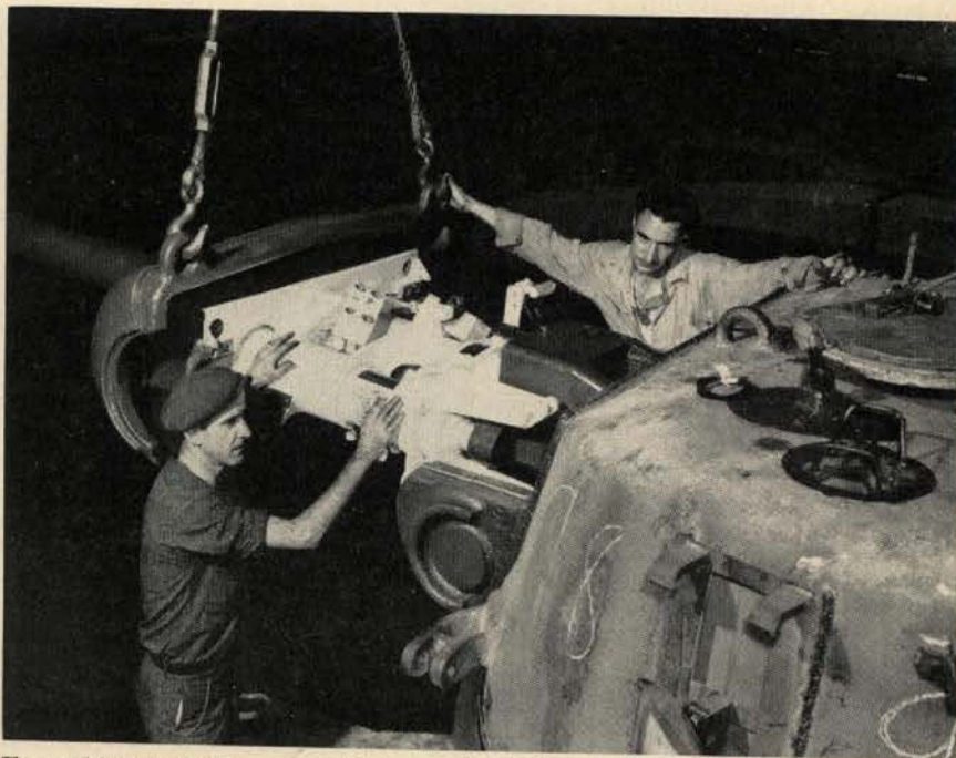
Everything is built around the gun. The 90mm assembly goes into a Patton.
