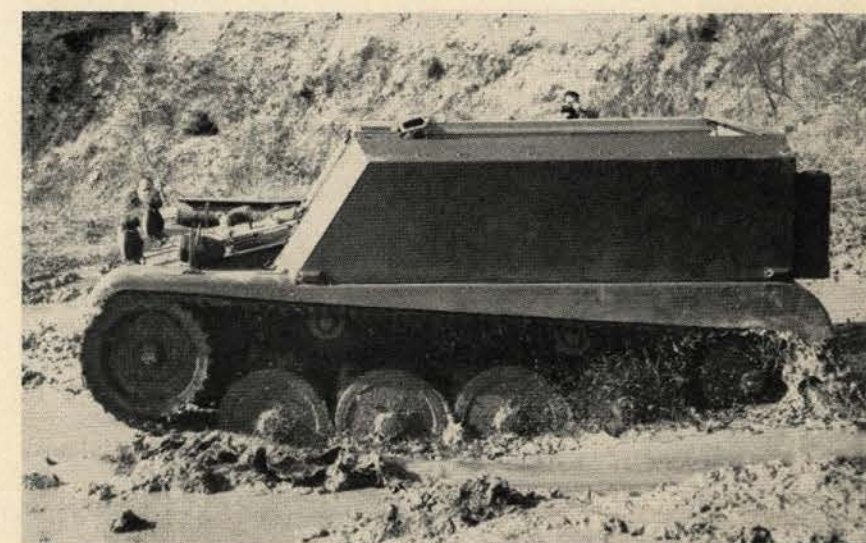
The new French Hotchkiss armored personnel carrier weighs 4 tons, carries six.
