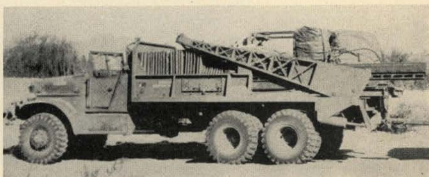
Engineer Bridge Truck carrying a float load.
