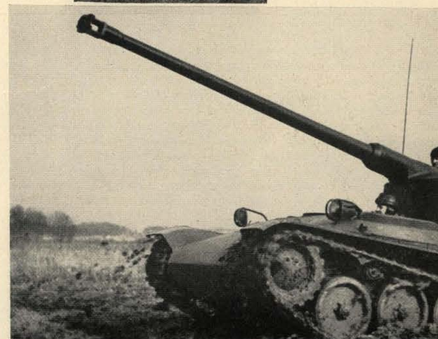
Variously described as a gun platform or tank destroyer, the new French light tank weighs 13 tons; crew 4; 75mm gun; 250 hp engine; height 6½'; speed, fast!
