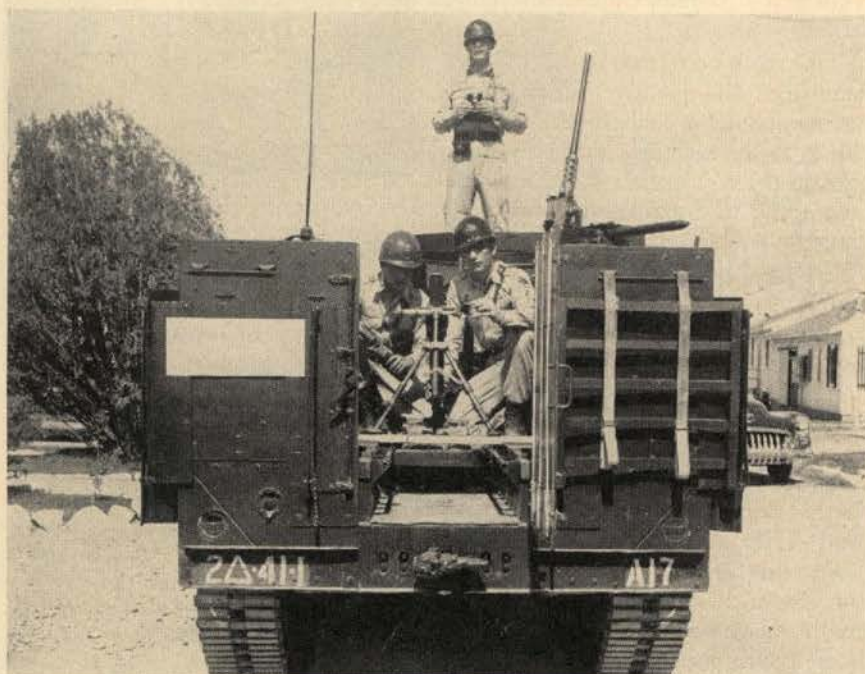
View showing the 60mm mortar mounted in half-track.
