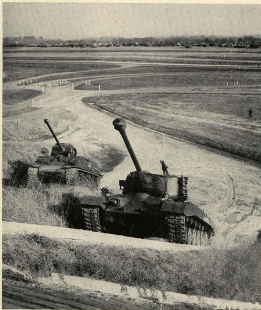
Testing on the proving ground. The Patton on a 40% grade outclimbs the Sherman on a 30% grade.
