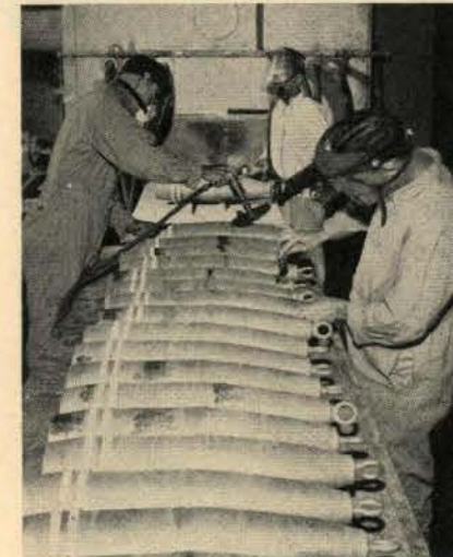
Ammo for the weapons. The original paint is sandblasted off, a new coat and stencils go on.
