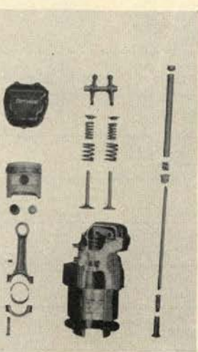
Figure 4 67 cu. in. cylinder and interchangeable parts.
