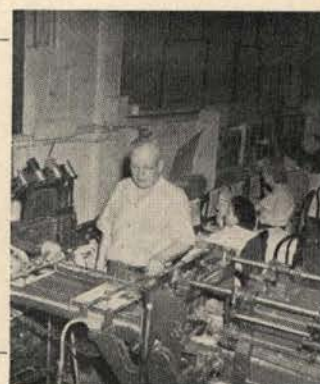
This is the Trimmer at the delivery end. Misses Spencer, Orange and Giddings are feeding signatures to the machine, while operator Vaughan checks the publication as it passes through the Trimmer. When the magazine reaches the delivery end of the Gatherer-Stitcher-Trimmer, it is ready for mailing.
