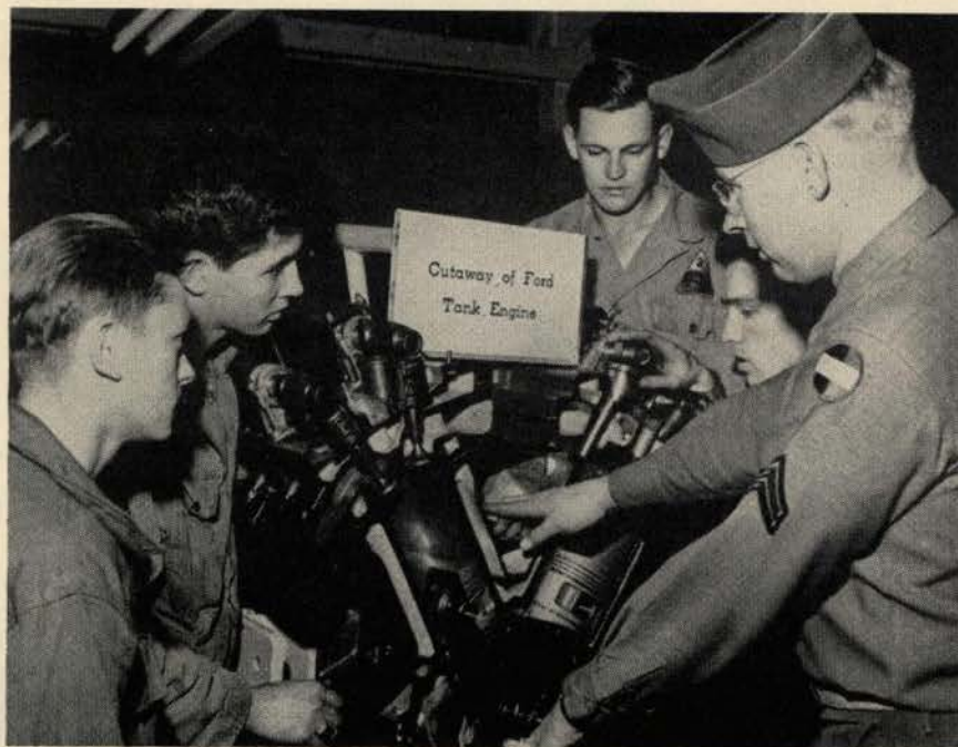
U.S. Army Tankers must know the mechanics of their vehicles. The functioning of the tank motor is well demonstrated by means of cutaway models at Ft. Knox.
