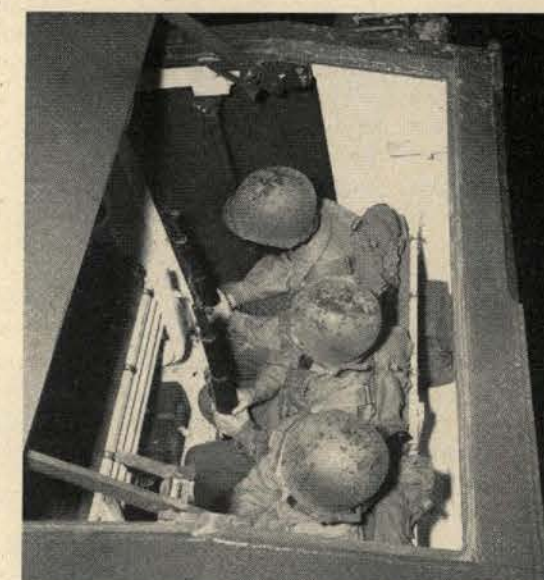
Side ports may be opened or put in semi-closed position and used by riflemen for close-in protection.
