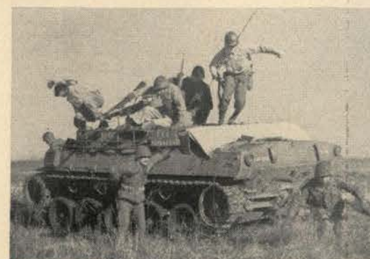
The M39 lacked important overhead protection.
