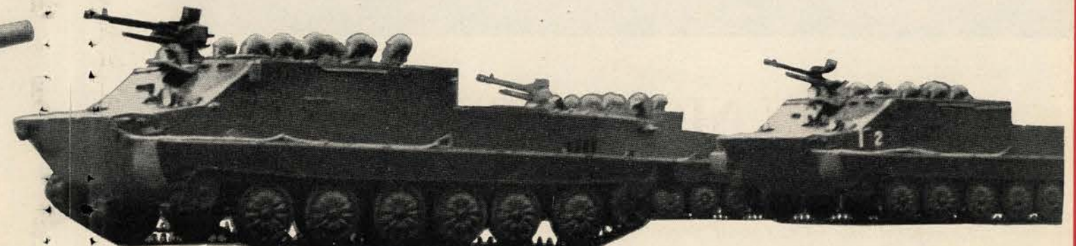
▲ The new amphibious APC. Its carrying capacity is approximately 15 men.
