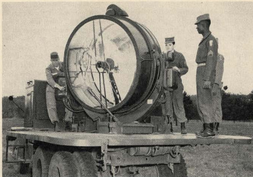
This is one of the two truck-mounted 60-inch searchlights that were used in the test. This light can be operational in 30 seconds from the time vehicle stops.
