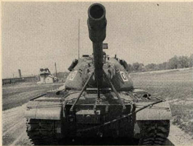
A rear view of the T43 heavy gun tank with its 120mm high velocity gun resting in the travelling position.
