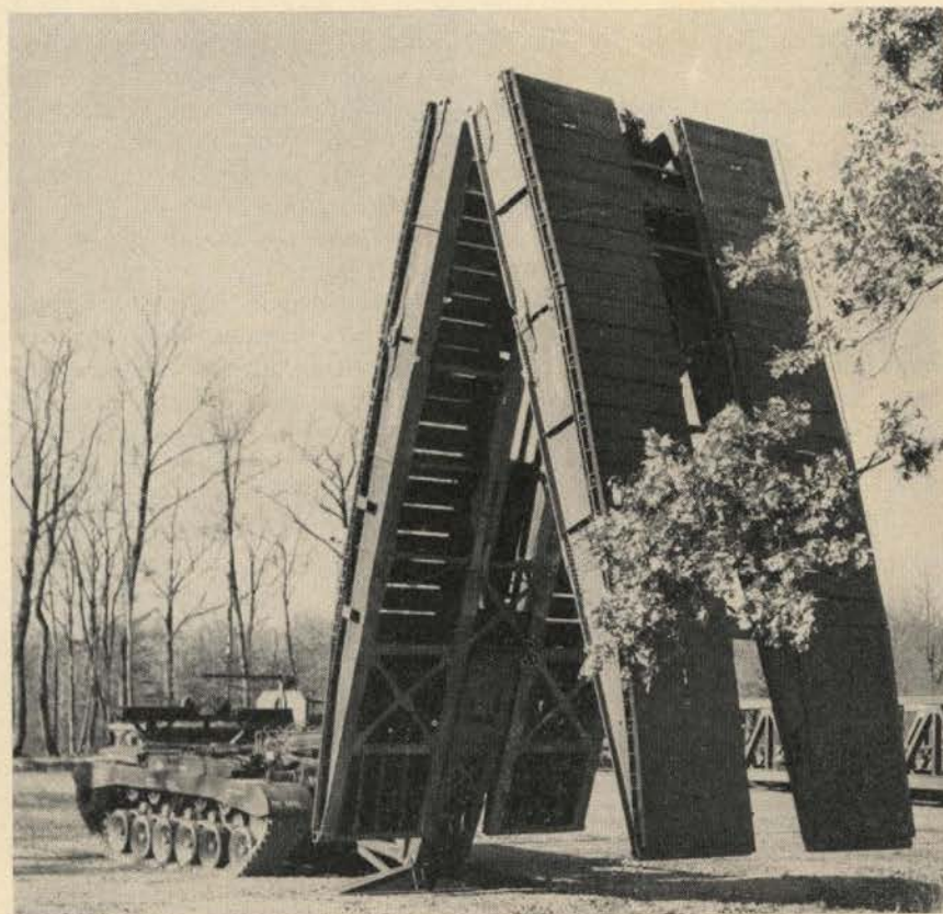
The Scissors-type, made of aluminum, commences unfurling at the launching site.
