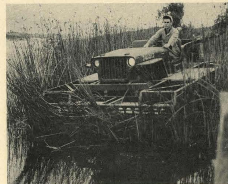
The "Rolligon" will negotiate terrain where a man on foot would bog down to his armpits, and it actually improves the ground over which it travels.
