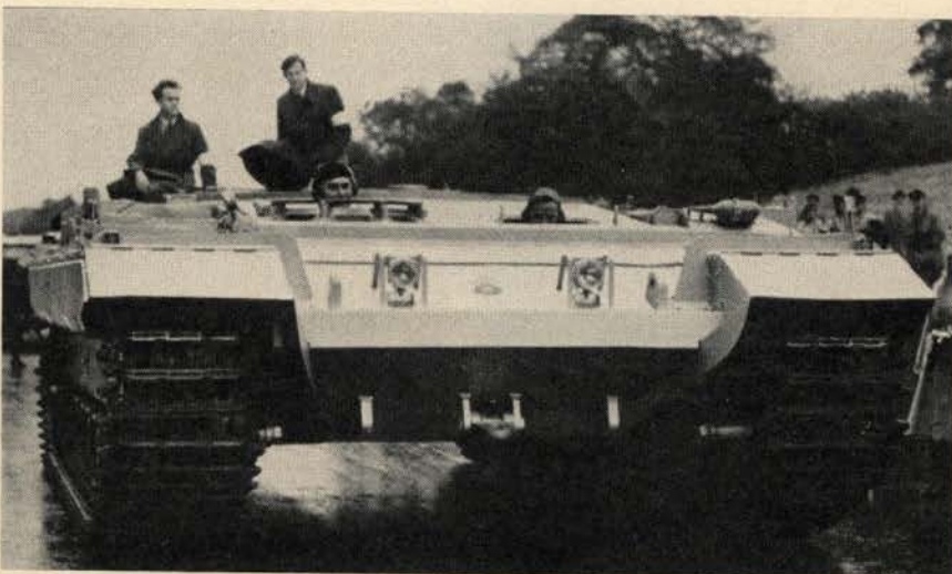
British Information Services The World's first gas turbine tracked vehicle, this British development is capable of 1,000 horsepower with a speed of 17,500 revolutions per minute.
