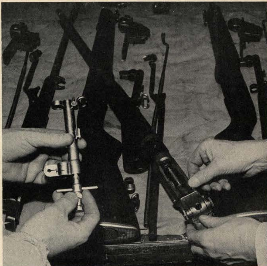
M1 rifle parts are meticulously gauged during Army Ordnance Inspection. U.S. Army
