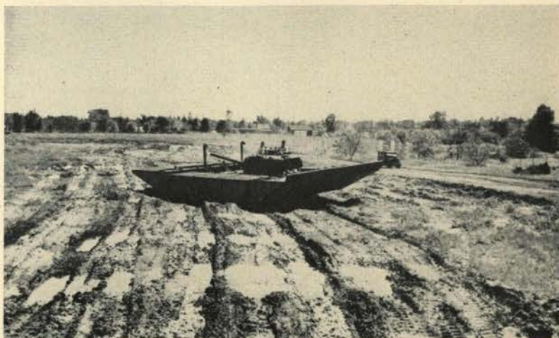
in deep water. The tank is capable of defending itself. In the lower photo, the floating device is shown on shore in position to jettison its pontoons.
