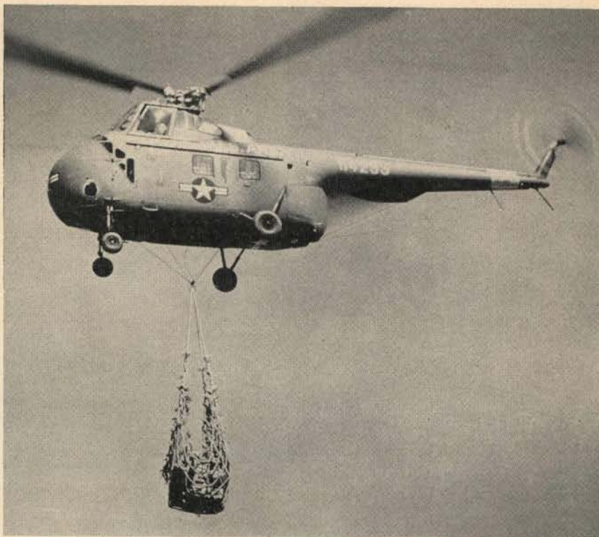
The H19 helicopter's limited capacity makes it unsatisfactory for fuel re-supply.
