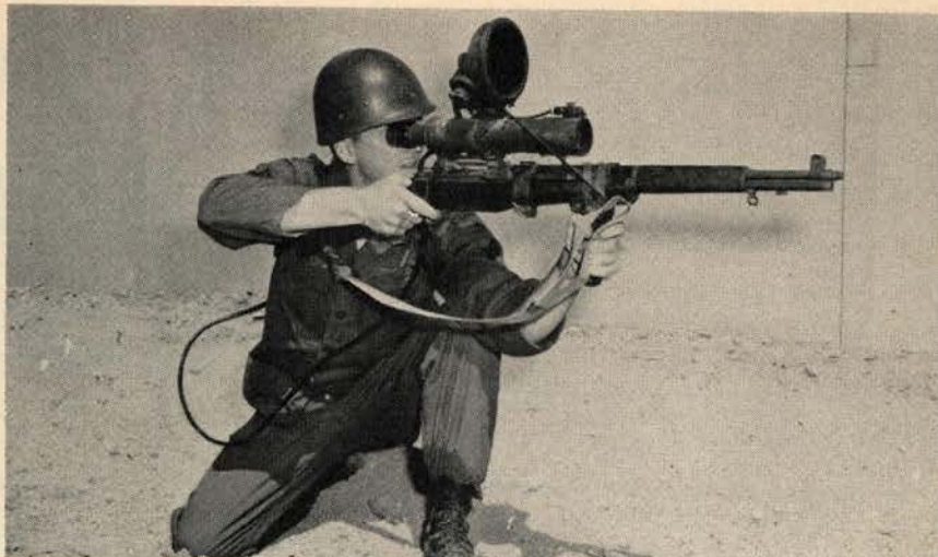
U. S. Army The new Sniperscope is an improved version of the World War II model. It has a longer range, more rugged construction and a more accurate aiming device.
