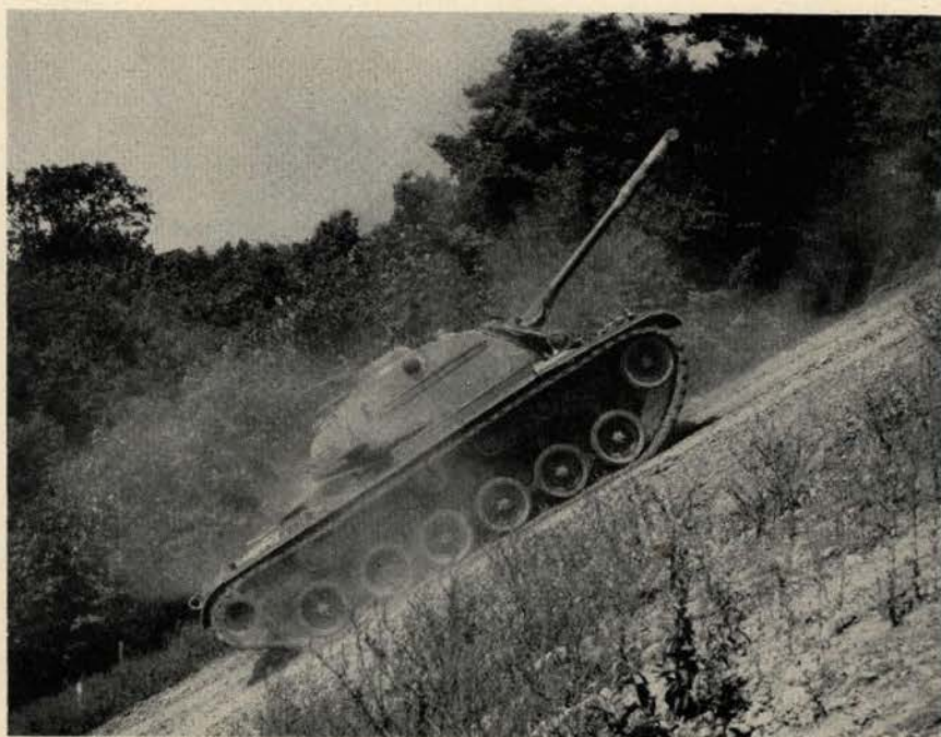
The Combat Vehicle Section testing a Patton 48 medium tank on a 60% slope.
