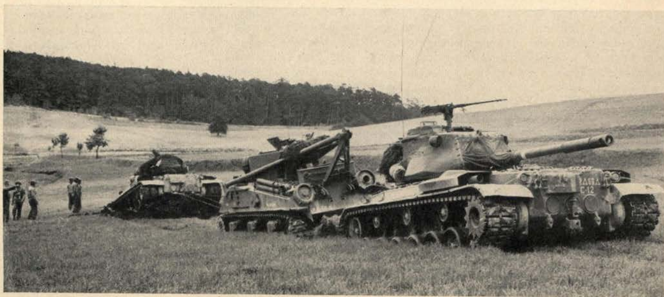
Bogged down in a deep mudhole, this tank is being put back into action by a tank retriever and a medium tank which have freed it from its predicament. A job which requires skillful teamwork saved this tank from falling into enemy hands.
