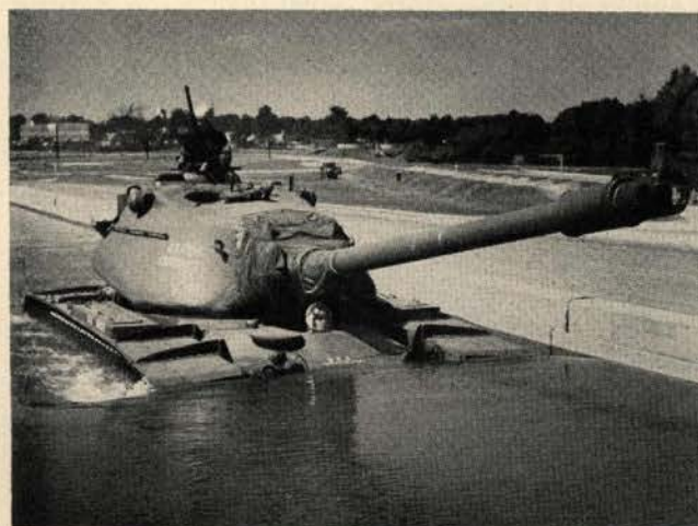
A low three-quarter view of the T43 moving slowly through the water bath basin at the Aberdeen Proving Grounds, Md.
