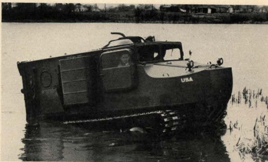
U. S. Army The M76 amphibious cargo carrier, the "Otter," is capable of traversing almost any type terrain at speeds up to 30 mph. It has a 135 horsepower engine.
