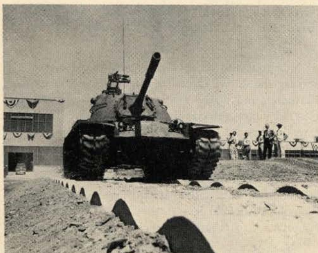
On a washboard the turret and gun ride smoothly, indicating the advantage to the gunner of scoring first rounds.
