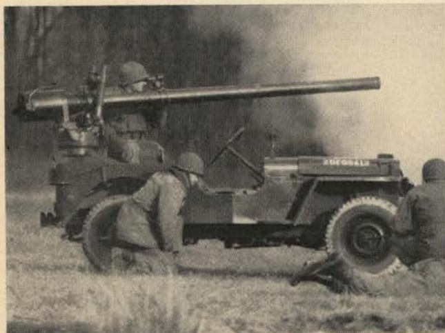
105mm recoilless gun mounted on a jeep. Limitations are a shorter range than tanks, no armor, and wheels, not tracks.
