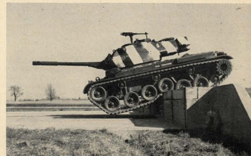
A test vehicle is put through the paces at Aberdeen Proving Ground where a rough course on tracks, suspension and power plant tests its maneuverability.
