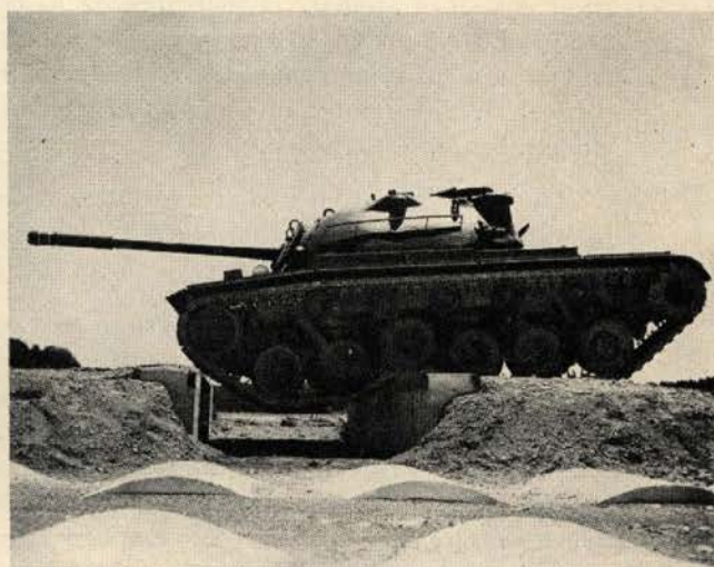
One of the tests of maneuverability is that of crossing an eight-foot trench. The T48 can negotiate some bad terrain.
