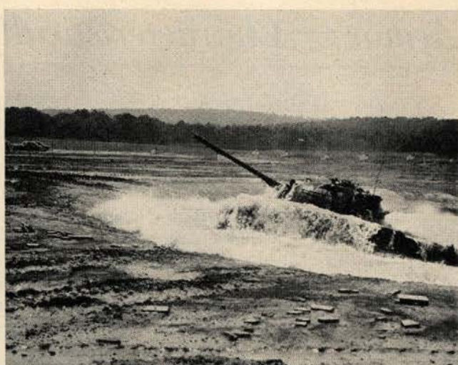
Shedding water like a surfacing submarine, the T48 emerges from a plunge that shows waterproof qualities.
