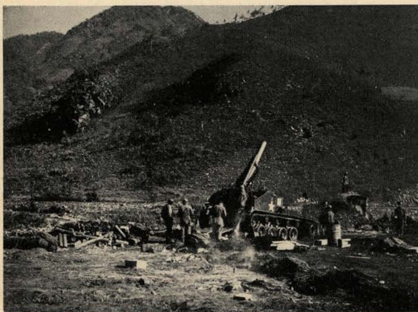
Certain limitation in ability to employ very high angle fire with the SP piece is offset by placing the vehicle on an appropriate natural or bull-dozed slope.
