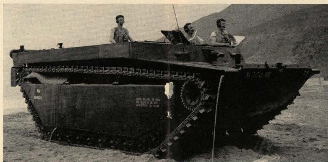
Amphibious Tractors comprise the second and subsequent waves in an amphibious assault on a hostile shore, transporting and landing assault elements of the landing force, and providing landing vehicles to transport personnel, equipment and supplies from ship to shore during the selective unloading of the build-up phase of an amphibious operation. They are unarmored.
