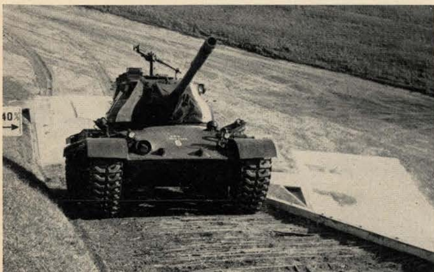
At Aberdeen Proving Ground the M47 is put through severe testing by Army Ordnance personnel. Here a test tank is required to prove itself on a 40% grade.
