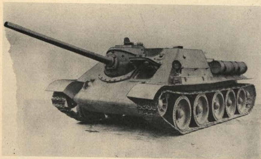
The SU-85 is a T-34 tank chassis and an M1939 85mm antiaircraft gun mounted.
