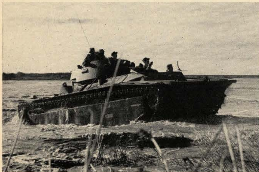
The amphibious tank mounts a 75mm and three .30s, and has a six-man crew.
