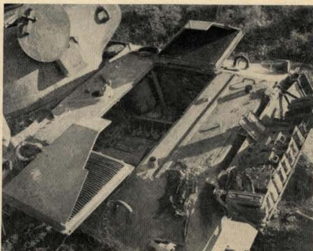
The fire leaves the engine compartment a mass of melted metal with exploded .30 caliber ammunition boxes outside.
