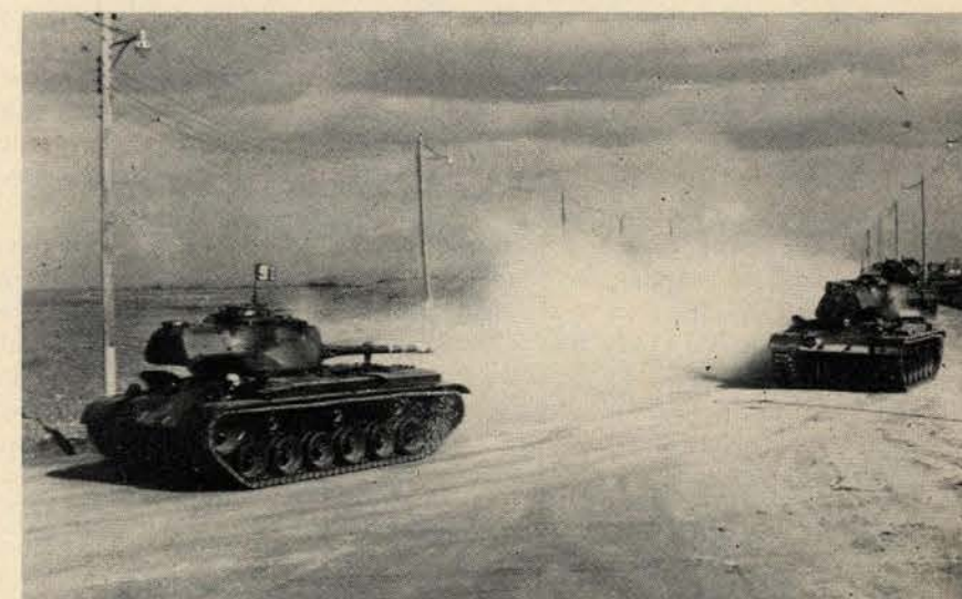
At the American Locomotive Company Plant in Schenectady, N. Y., each tank coming off the line receives a 45-mile "shakedown" before Ordnance gets it.
