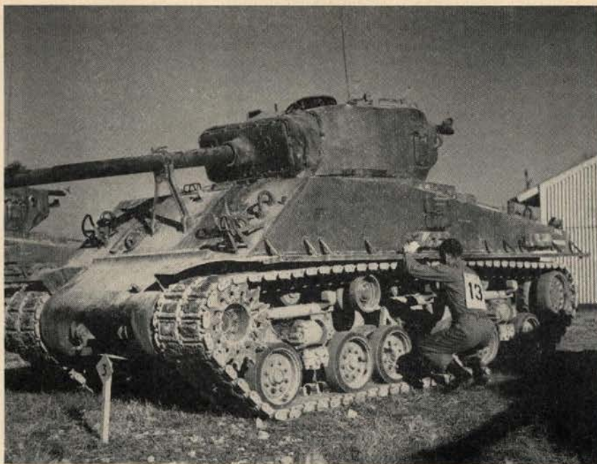
Meeting a problem in 1st echelon tank maintenance at this station, contestant must determine the correctness of track tension on this M4A3E8 Sherman tank.
