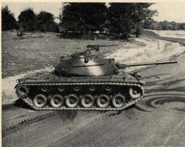
Tracks tell the story—that the new tank is capable of pivoting within its own length, a key feature in maneuvering.
