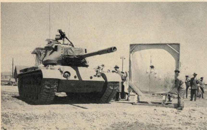
To tankers the armament is the key item. Here's the kind of shot pattern turned in by the M47's 90mm high velocity gun firing at a target at an 800-yard range.
