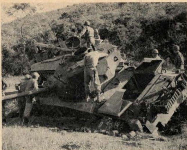
Surveying the recovery problem. Members of the maintenance platoon pass a towing cable around the tank turret.
