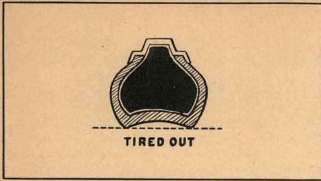
Tired out—Overloading has the same effect on tires as underinflation. Distortion of casings breaks them down. Treads wear quickly and unevenly.
