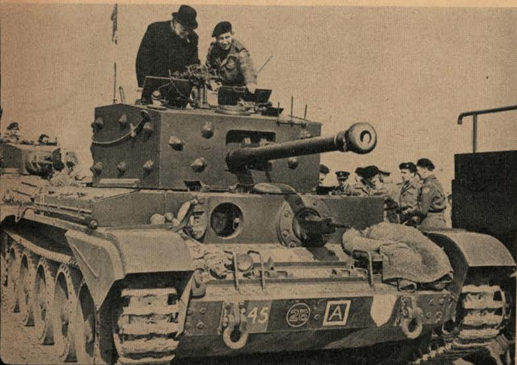
The Cromwell tank, which made its debut in Normandy, is one of the latest types of British cruiser tanks. It incorporates a 75mm gun and a high capacity British engine. It proved to be a most reliable and effective addition to British armor on the Normandy front. This picture was taken during a visit of Mr. Churchill to British troops in Britain and shows the Prime Minister inspecting a Cromwell tank.
