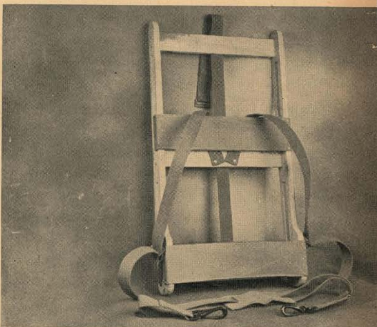
Type No. 1. Two-man pack. Back of frame shows web back bands and adjustable harness. Note attachment. Front of pack frame shows recess for set unit and method of attaching lashing strap. Lashing strap is inserted through slots, buckle end to top.
