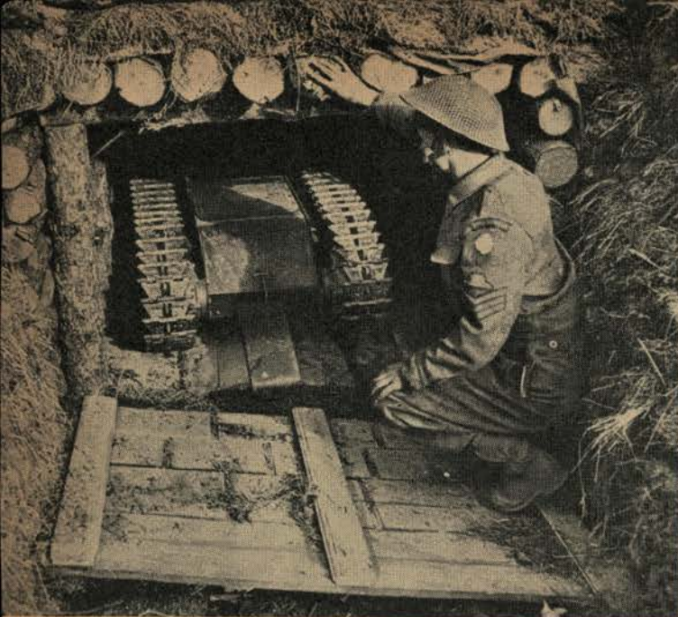
A British soldier looks at a captured German Goliath or "doodlebug" found recently in a dugout in the Normandy beach area of France. First used on the Anzio Beachhead, this type of weapon, carrying a heavy explosive charge and operated by remote control, is not retrievable.
