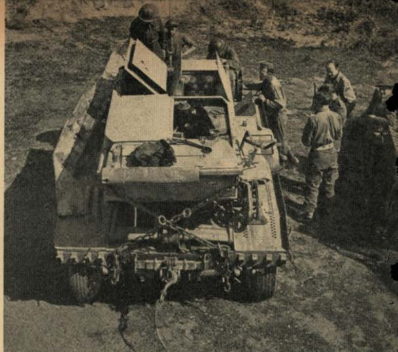
This radio-controlled "tank," called by the Germans the B4, is an explosives carrier. Above picture was taken looking down on the tank from the rear. This was recovered with great difficulty, under enemy fire. Unlike the "doodlebug," it can be recovered after demolition is dropped.
