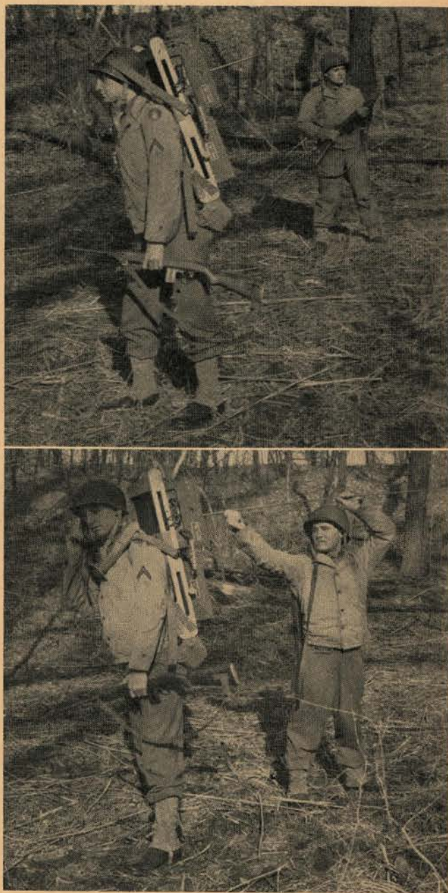
Top. One-man pack. Load is carried high and well balanced. Attachment and adjustment of tump line are shown. Bottom. Tump line is dropped to chest during transmission and for rest. Station can be put on the air quickly.
