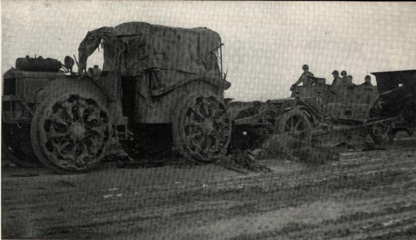
This Italian 105mm field howitzer with its tractor was captured by rapidly advancing American troops in Tunisia. The tractor wheels are equipped with grousers that roll out for use in deep mud or sand. In background (behind gun) is the U. S. armored car that made the capture.
