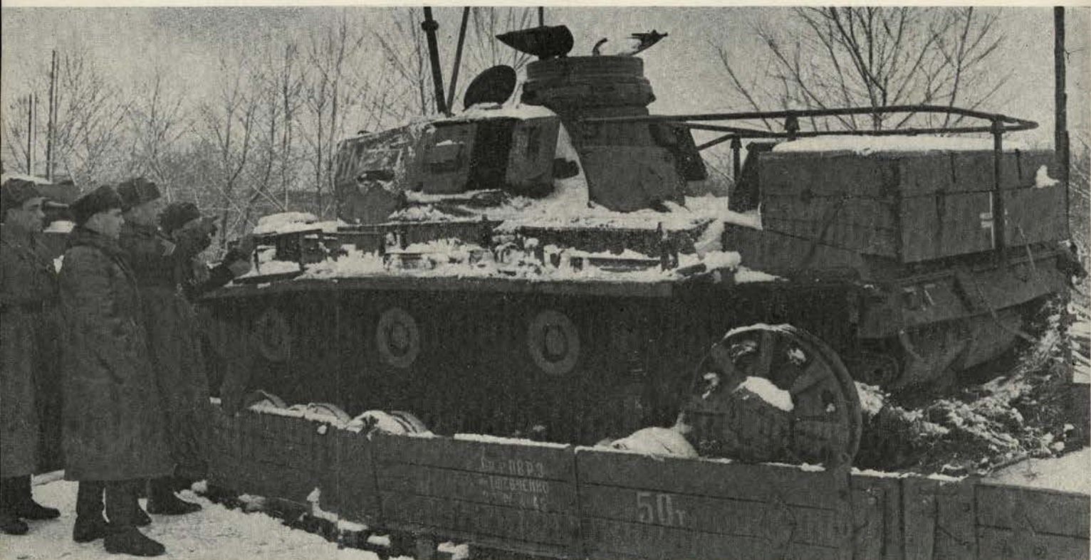
This Mark III tank, captured on the Southern Front, is off to the factory for repair. It is identified as a command tank because of its two radio aerials, one looking like a railing on the rear of the tank, and the other standing out above the turret. Armament consists of one 50mm gun on the newer models and a 37mm gun on the older ones. A dummy gun helps to conceal its command function.
