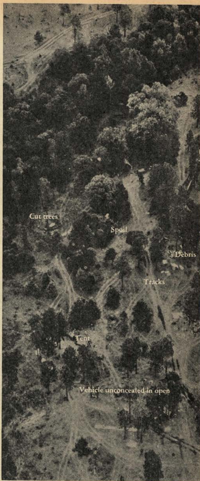
Fig. 1. Signs of military activity often give away valuable clues to the existence of an installation. Some typical examples of revealing traces are shown above. Tank tracks are different than those of other vehicles, hence, the presence of an armored unit in an area may be determined by these tell-tale traces alone.
