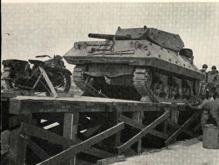
Figure 3—Details of blocking and securing of motorcycle and M-10 Destroyer as completed by OC students. No. 5 patterns (padded) are used on cycle wheels, and Nos. 2 and 3 on M-10. Note inexpensive construction of "TDS-RR."
