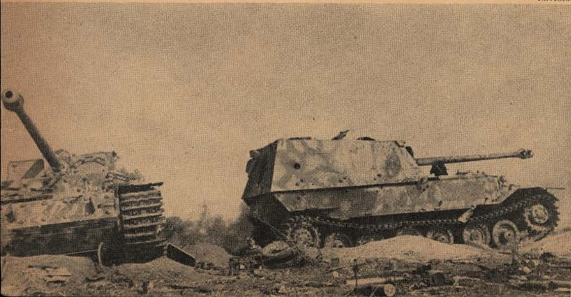
These 70-ton "Ferdinand" tank destroyers (mounting 88mm gun) were captured on the Orel front. Armor runs from about 8 inches in front to 3 inches in rear. The "Ferdinand" has two 300 h.p. motors, makes about 12 m.p.h. on a highway, and carries a crew of six. It is steered by periscope; must stop to fire. Hole in side of right vehicle is observation post; plug sealing it is missing. Poor visibility for crew makes this new German weapon particularly vulnerable to attack by infantry.
