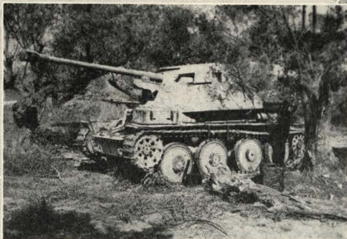
PzKw38t (1938 Czech tank chassis) with F K.36R—the Russian M1936 high-velocity 76.2 mm field gun.
