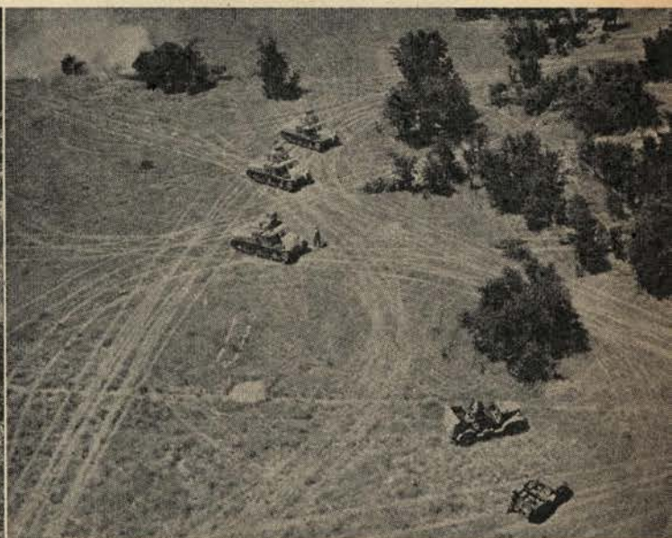
Fig. 10. Result of uncontrolled track plan. Ninety per cent of these tracks could have been avoided. Concealment measures following this are futile.
