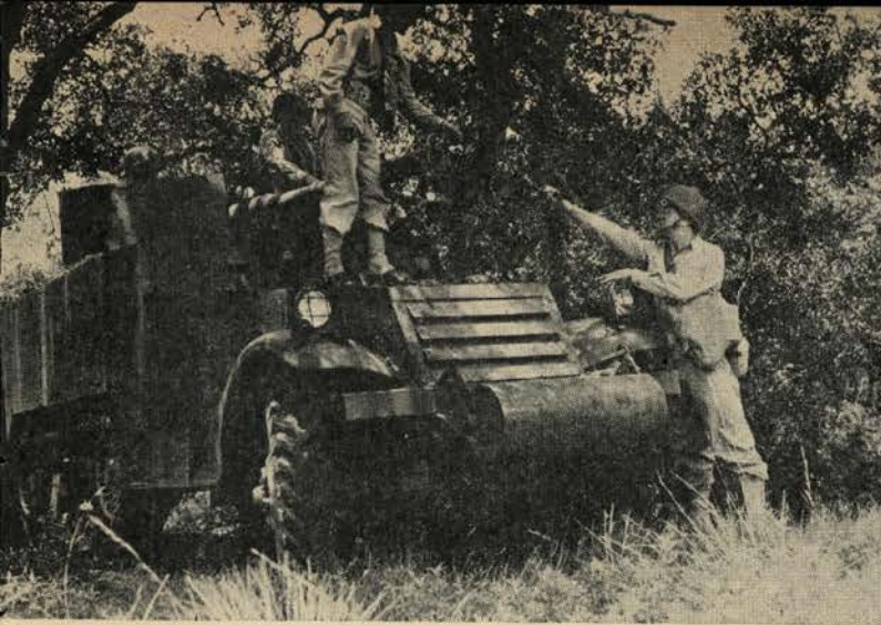
Fig. 3 and 4. Before and after. Outline, shadow, and reflections are broken up and concealed with natural materials.
