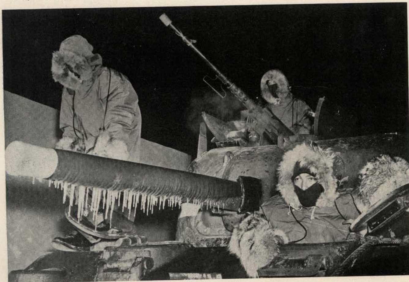
Sub-zero temperatures in the cold-room of the laboratory are graphically shown by the ice on this tank and the bulky, but comfortable, clothes of the Armored Force emerging from this M-4 tank. Experiments in this room are usually conducted at 30 degrees below zero.
