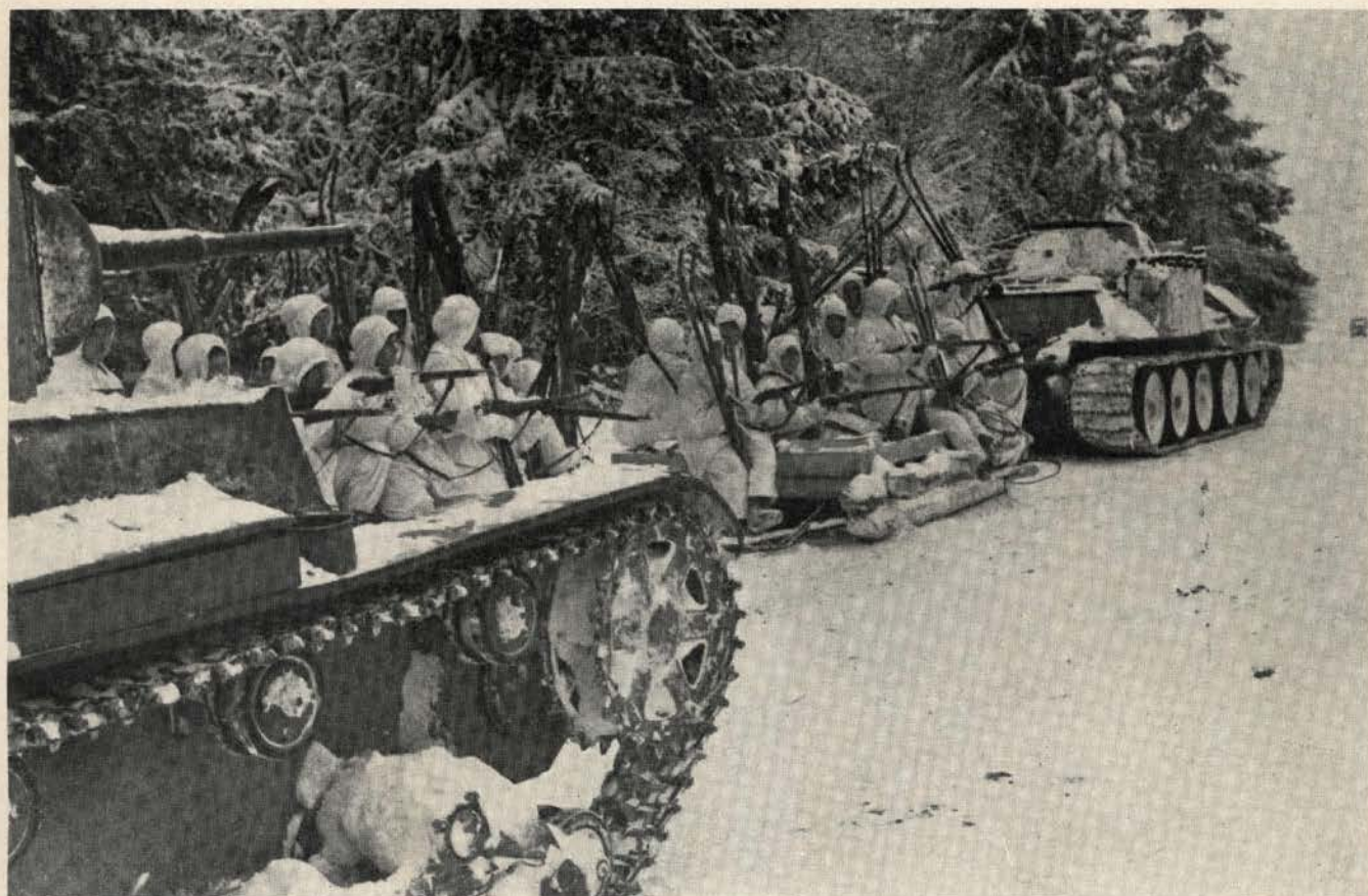
"The armored sleigh, without any firing power of its own, is towed by the tank to the forward edge of the enemy's defensive zone. Then the sleighs are unhitched and the infantrymen, supported by the fire of their tanks, dismount and go into action."
