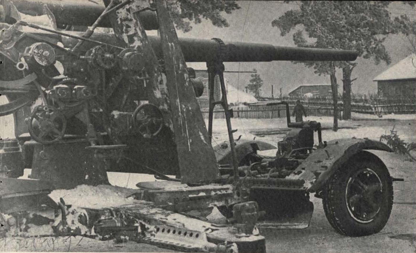
This German 88mm dual-purpose gun, captured by the Russians during their winter drive, is of the type that has been used effectively both in Africa and on the Russian front. It was also used in 1940 to smash the bunkers of the Maginot Line. Note the elevating and traversing mechanism which makes it both an antitank and antiaircraft gun.
