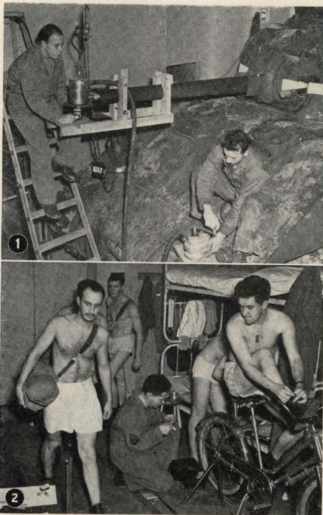
1—In important gun-fume tests, gas is pumped through the gun barrel of this 75mm cannon into an M-4 tank. Tests then discover the effectiveness of the tank's ventilation system in removing harmful gas fumes. 2—Several experiments are conducted simultaneously within the hot-room. While three men plod their way around the room with a forty-pound pack, another prepares to mount a stationary bicycle and pedal in place for a ten-minute period.
