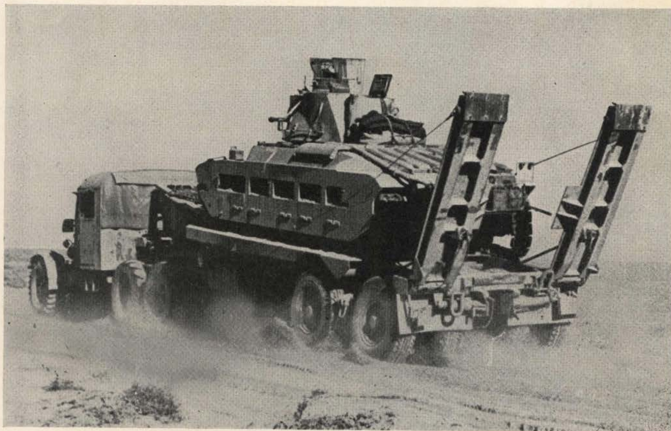
Tank maintenance must go forward on schedule, even in the desert. The tank transport is hauling a 26-ton British tank.
