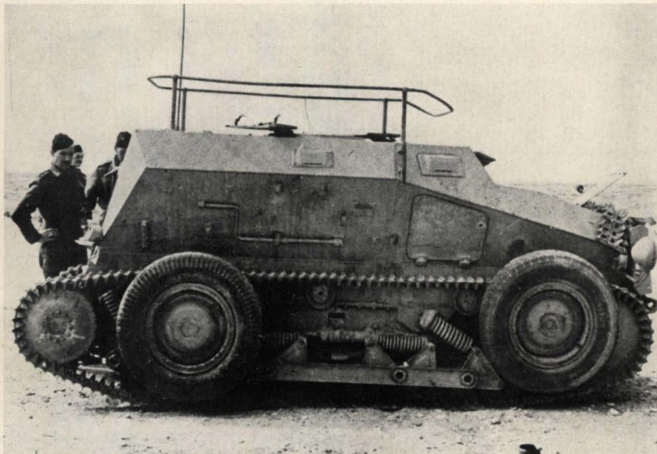
A Nazi half-track armored observation car captured by the British. This car is so equipped that where speed over level terrain is desirable, the tractor tread can be raised and the tired wheels lowered to provide the traction.
