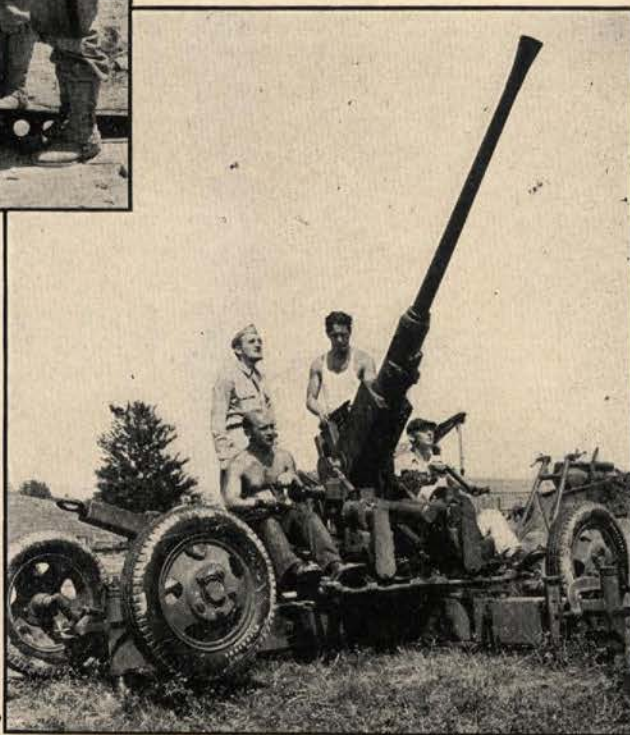
Below: One of the first of the new Bofors to come off assembly lines. This 40-mm. gun, developed first in Sweden, is now standard in British, United States armies.
