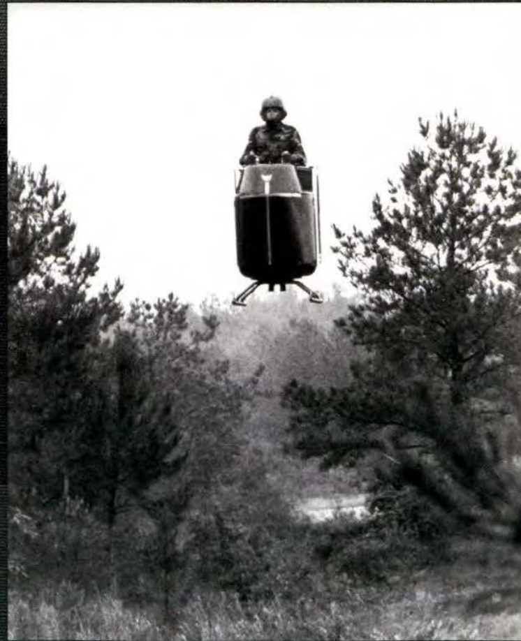
Above, the WASP II (Williams Aerial Systems Platform), an experimental aircraft powered by a turbofan engine, could take off vertically and fly for 30 minutes at speeds up to 60 mph. Though never used in service, test flights were conducted at Fort Benning by infantry soldiers without piloting experience under a contract to the U.S. Army Tank Automotive Command (TACOM), June 18, 1982.
