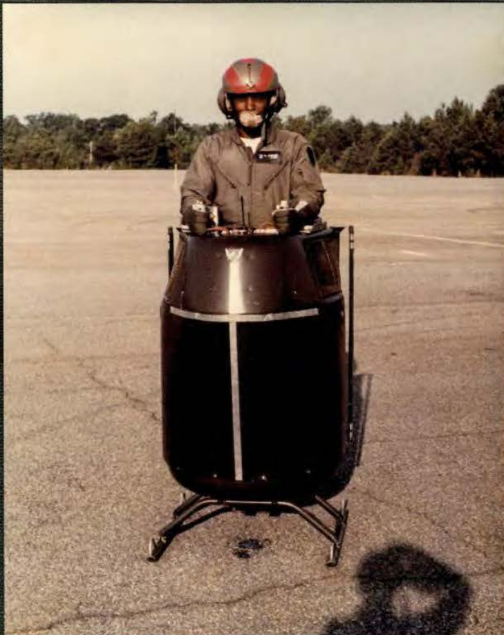
Above, the WASP II (Williams Aerial Systems Platform), an experimental aircraft powered by a turbofan engine, could take off vertically and fly for 30 minutes at speeds up to 60 mph. Though never used in service, test flights were conducted at Fort Benning by infantry soldiers without piloting experience under a contract to the U.S. Army Tank Automotive Command (TACOM), June 18, 1982.
