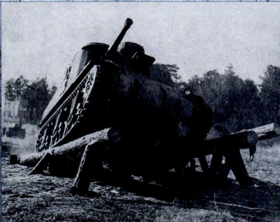
An M3 Lee Tank attempts to breach an obstacle emplaced by the 55th Engineers, Fort Benning, 1943.
