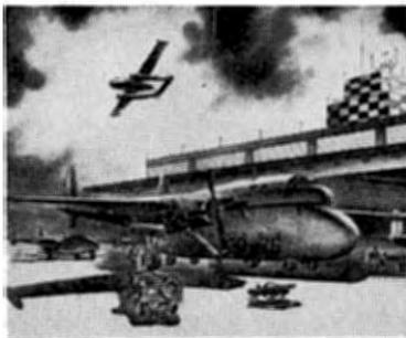
The C-120 shown at left and on the cover will be the first plane to apply fully the principles of the trailer truck to an airplane. It will fly with or without its fuselage, a factor permitting easy ground handling of supplies and at the same time provide storage units. This photo and the one on the bottom of page 12 are through the courtesy of the Fairchild Aircraft Co.
