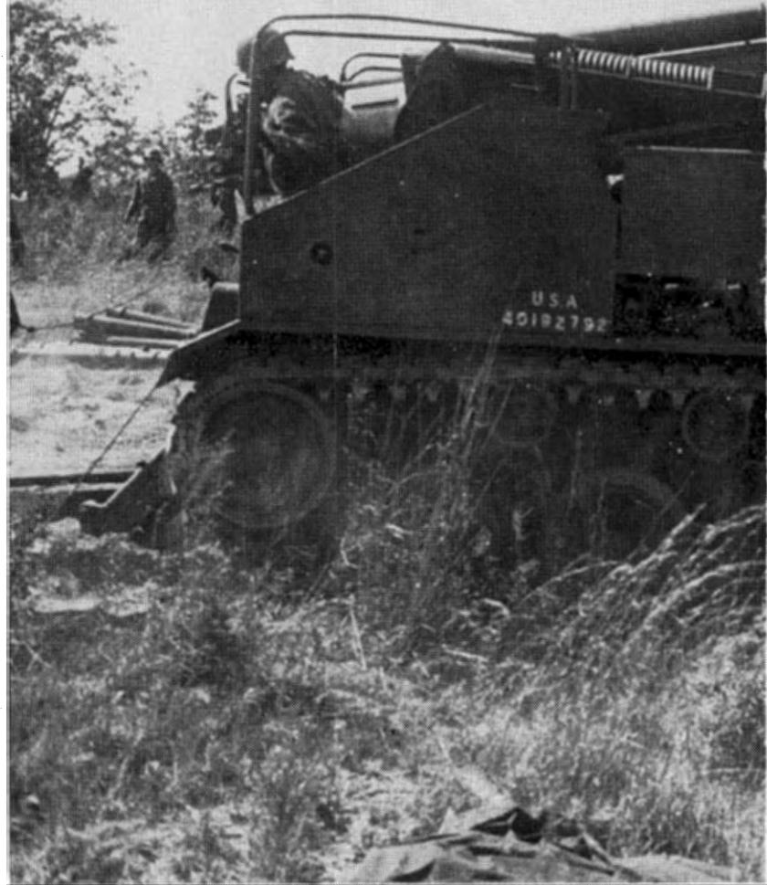
THE M-41S OF THE 999TH, SHOWN HERE, HAVE A MAXIMUM RANGE OF 16,350 YARDS. DEVELOPED DURING WORLD WAR II, THEY WEIGH 42,000 POUNDS, CAN MOVE AT 45 MILES AN HOUR, CARRY 32 ROUNDS OF AMMUNITION AND CAN FIRE AT THE RATE OF THREE
